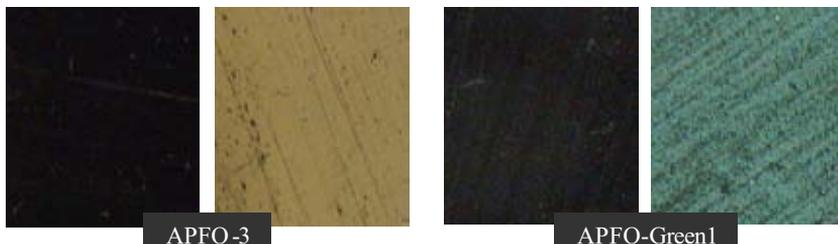
Figure 8.3 Birefringence observed under an optical microscope equipped with crossed polarizers. The colored monographs were recorded at a  $45^\circ$  angle difference with the dark ones.
