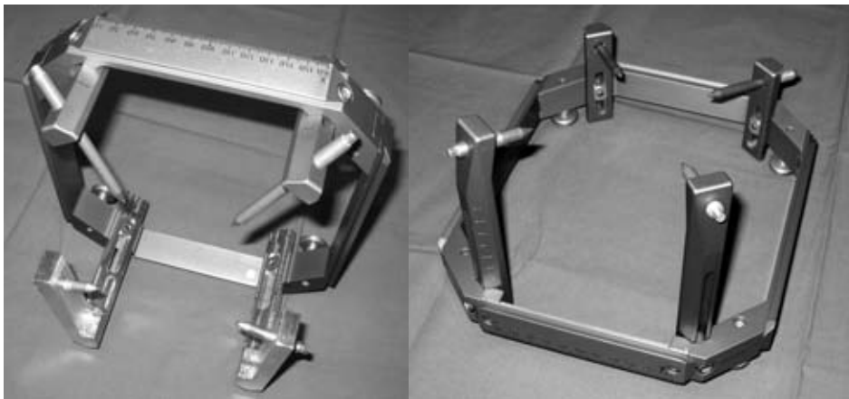
Figure 7. Example of the modification on the stereotactic frame. a) Modified posts for the porcine skull, b) unmodified human frame.
