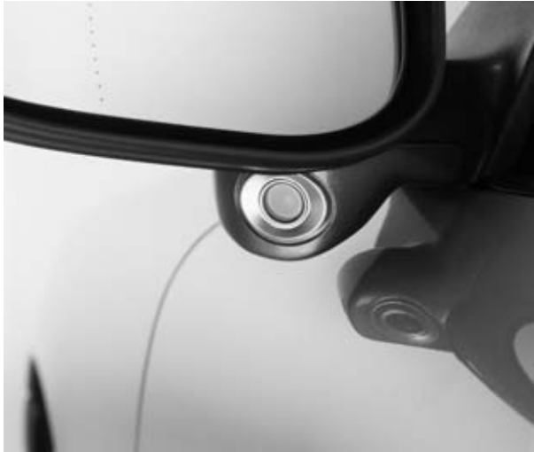
Figure 2.2: The Volvo Blind Spot Information System (BLIS). Photo: Volvo Car Corporation.
