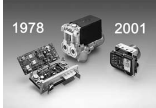
Figure 2.1: 1978 and 2001 ABS unit. The 2001 system is much more compact. Photo: Bosch
