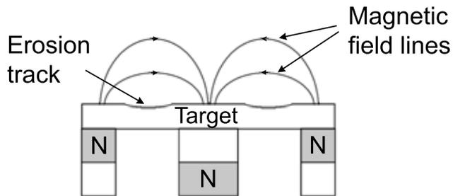
**Figure 3.** Schematic drawing of a magnetron.
