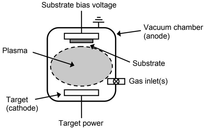
**Figure 1.** Schematic drawing of a simple sputter deposition system [13].
