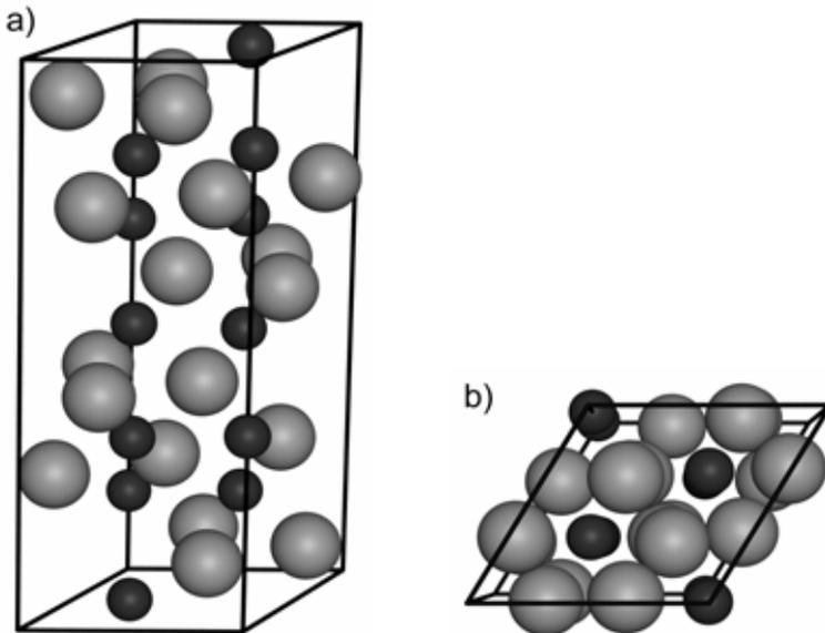
**Figure 8.** Side view (a) and top view (b) of the hexagonal unit cell of  $\alpha$ -alumina. The smaller, darker spheres represent aluminum atoms and the larger, brighter ones oxygen atoms.
