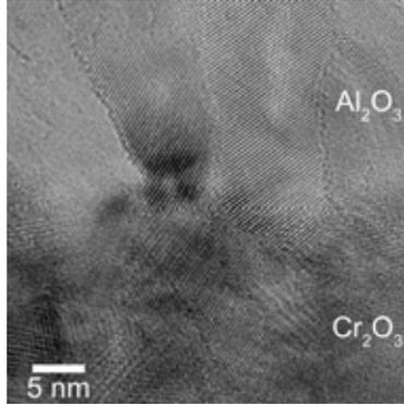
**Figure 7.** Cross-sectional high resolution transmission electron micrograph of a  $\text{Cr}_2\text{O}_3/\alpha\text{-Al}_2\text{O}_3$  interface. From Paper III.
