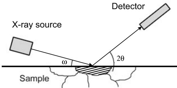
**Figure 6.** Schematic illustration of an x-ray diffraction setup.
