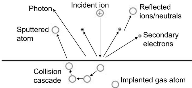
**Figure 2.** Different possible processes occurring at the target surface.
