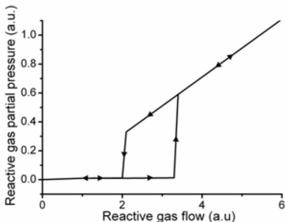
**Figure 4.** Typical hysteresis behavior of the reactive gas partial pressure as the reactive gas flow is varied.
