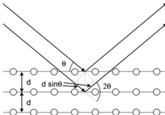
**Figure 5.** Schematic illustration of diffraction according to Bragg's law.
