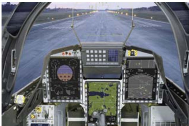
Figure 3. The glass cockpit of JAS 39 Gripen fighter aircraft. Photo from Saab AB.
