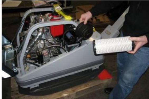
*Figure 14. The adapted air filter in FB-455 soil compactor.*
