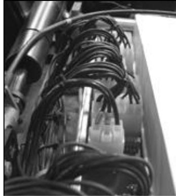
*Figure 9. Improper angle of insertion and position of electronic sockets facilitating dirt and water collection without any zones of drainage.*
