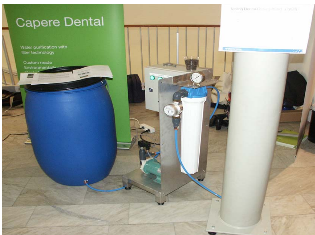
Fig.2 Capere Dental Separating Unit, cotton filter to the right, bark container on the left, photo by the author.
