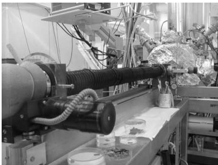
Figure 6.2 The photoelectron spectrometer "Moses"
