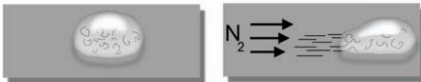
4.2 Schematic illustration of molecular combing (moving air-water interface). (Left) A droplet of liquid with wire-like molecules in a more or less coiled geometry is deposited on a surface. The molecules have a weak affinity to the surface. (Right) The droplet is moved along the surface, e.g. using a directed gas stream. The molecules are elongated perpendicularly to the moving air-water interface and left stretched on the surface.
