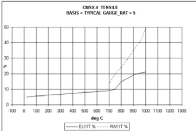
**Figure 3.3:** Tensile elongation of CMSX-4 at different temperatures for CMSX-4 (by courtesy of Mick Whitehurst, Siemens, Lincoln, UK). EL11T is elongation in % and RA11T is reduction of area in %.
