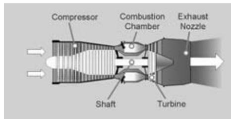
**Figure 3.1:** Illustration of the basic components of a simple gas turbine engine [10].
