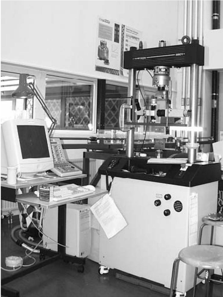
**Figure 3.16:** Equipment used for both low cycle fatigue and thermo-mechanical fatigue tests.
