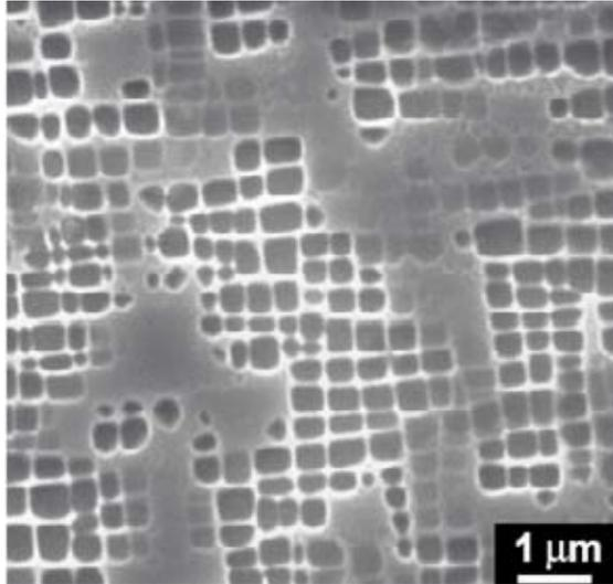
**Figure 3.6:** Cubical  $\gamma'$  precipitates in SCB after fully heat treatments at 1270°C/4h and 1100°C/4h, [16]
