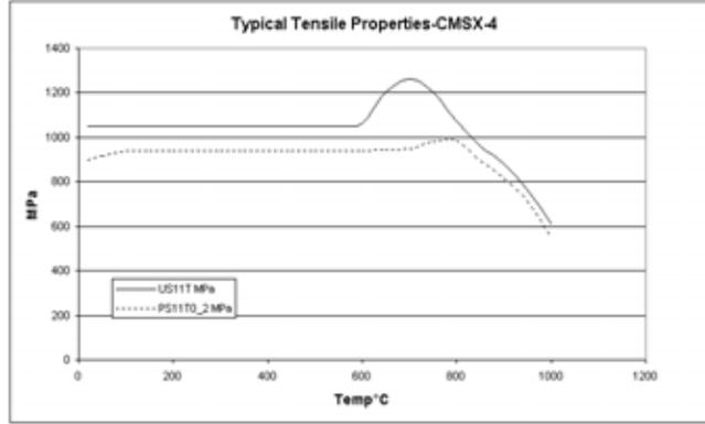
**Figure 3.2:** Tensile properties of CMSX-4 at different temperatures (by courtesy of Mick Whitehurst, Siemens, Lincoln, UK). US11T is ultimate strength in MPa, PS11T0.2 is yield strength in MPa.
