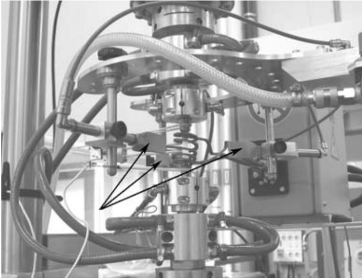
**Figure 3.17:** Set-up of a thermo-mechanical fatigue tests. The arrows show the nozzles used during cooling cycles.
