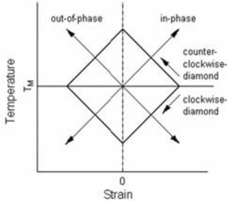
**Figure 3.14:** Strain and temperature variations for different TMF cycles [44].
