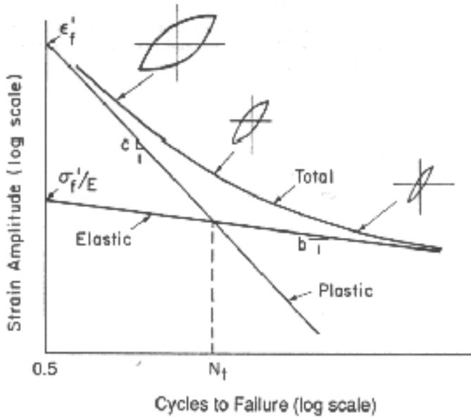
**Figure 3.12:** Strain-life curves showing total, elastic and plastic strain versus reversals failure.
