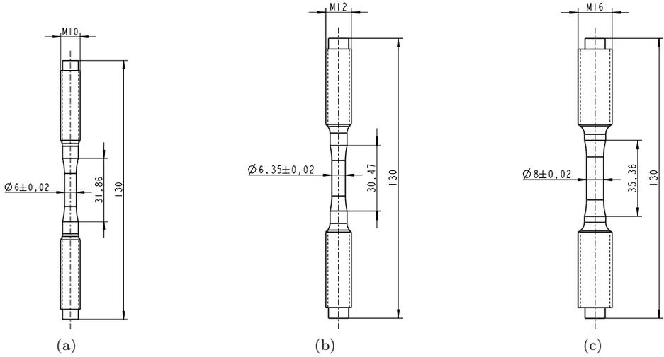
**Figure 3.15:** Low cycle fatigue, a and b, and thermo-mechanical fatigue, b and c, solid specimens used in the experiments.
