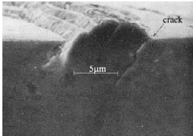
**Figure 3.13:** Fatigue crack initiation in a copper crystal,[33].
