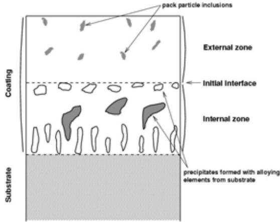
Figure 3.10: Typical microstructure of an aluminide coating, [25].
