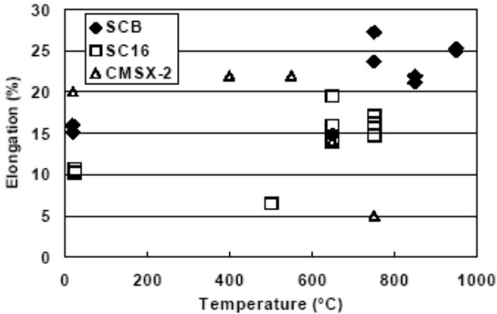
Figure 3.9: Elongation of SCB at different temperatures, [16].
