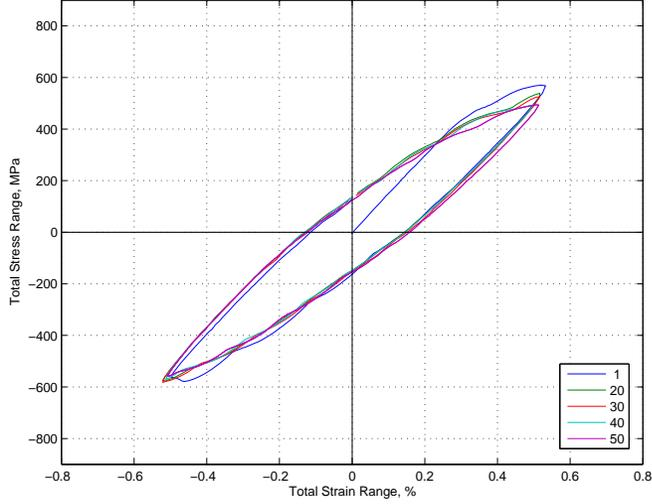
**Figure 3.11:** An example of a hysteresis loop obtained for IN792 tested at 900°C and a strain range of 1%.
