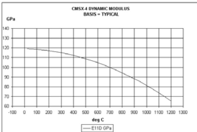
**Figure 3.4:** Dynamic modulus of elasticity for CMSX-4 at different temperatures (by courtesy of Mick Whitehurst, Siemens, Lincoln, UK). E11D is Young's modulus in GPa.
