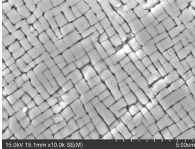
**Figure 3.5:** SEM micrograph showing microstructure of CMSX-4 after aging treatment at 1140°C/4h with uniformly distributed cuboidal  $\gamma'$  precipitates in  $\gamma$  matrix
