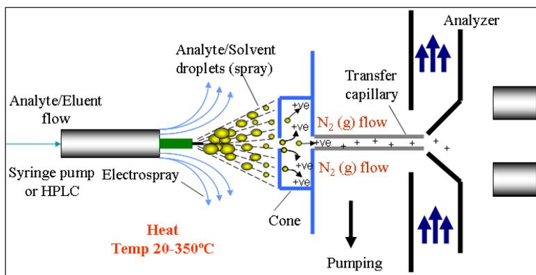
*Fig. 15 Schematic view of Electrospray Ionization MS*
