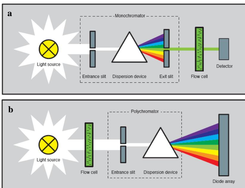
*Fig. 14. Schematic view of UV and PDA Detection principles*
