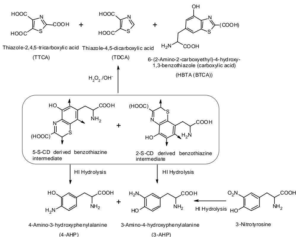
**Fig. 9.** Chemical degradation of pheomelanin
