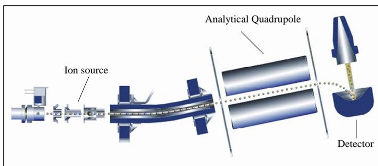
*Fig. 16. Schematic view of a quadrupole MS*
