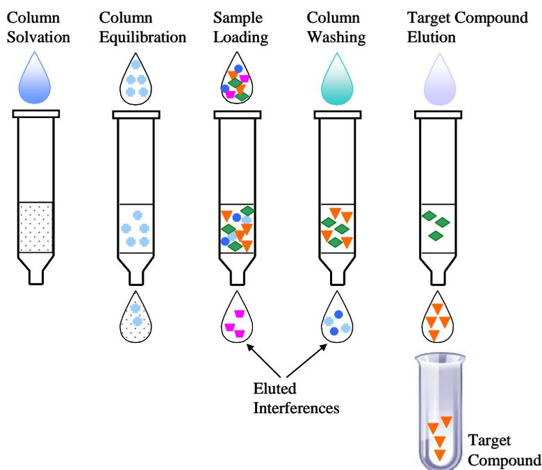
*Fig. 10. Schematic view of solid phase extraction procedure*
