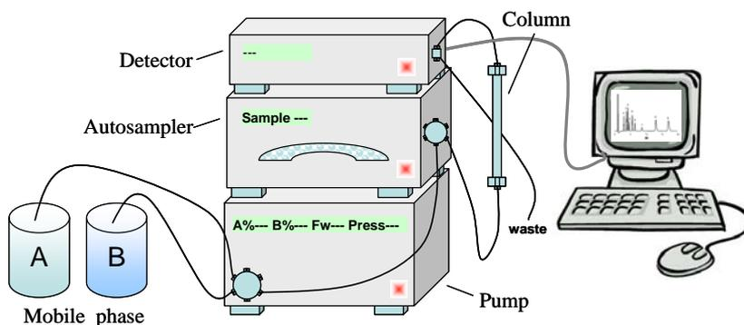
*Fig. 11. Typical scheme of an HPLC system*
