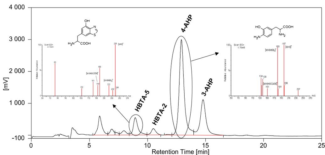
**Fig. 20.** Chromatogram of 4-AHP and 3-AHP from 1 mg synthetic pheomelanin. Detection was performed by ECD at +700 mV. A hitherto unidentified compound was identified as hydroxybesothiazole by LC/MS/MS.
