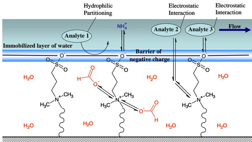
*Fig. 13. The retention processes in ZIC-HILIC illustrated by hydrophilic partitioning and electrostatic interactions with either positive or negative charges*
