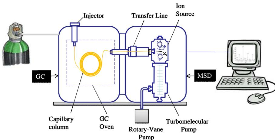
*Fig. 12. Typical scheme of a GC/MS system*
