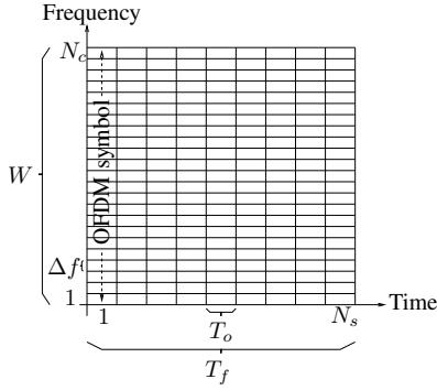
Fig. 1. OFDM time/frequency resource grid
