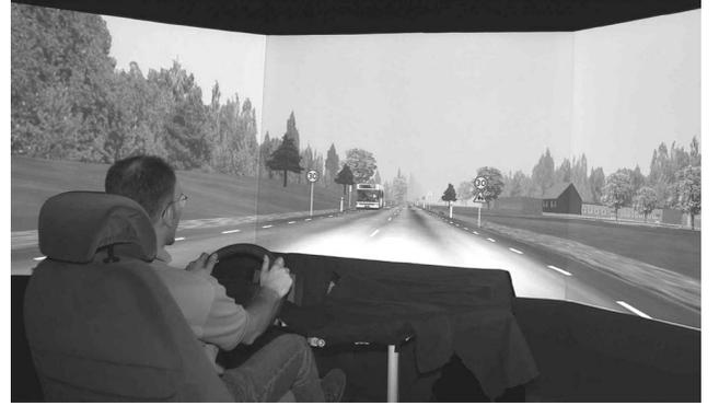
Fig. 3. The fixed-base driving simulator used in our study is software-oriented and allows for rapid prototyping of new driver assistance systems and HMI-features.
