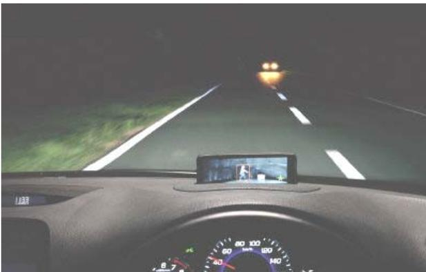
Fig. 1. NVS provide an enhanced view of the road ahead. The example shows Honda's intelligent NVS, which has detected a pedestrian. The system warns the driver by highlighting the pedestrian on the head-up display and by blinking an icon and sounding an alarm (more information can be obtained from Honda's web-site, [10])
