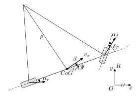
Fig. 2. Illustration of the geometry for the single track model, describing the motion of the host vehicle. The host vehicle velocity vector  $v_x$  is defined from the CoG and its angle to the longitudinal axis of the vehicle is denoted by  $\beta$ , referred to as the float angle or vehicle body side slip angle. Furthermore, the slip angles are referred to as  $\alpha_f$  and  $\alpha_r$ . The front wheel angle is denoted by  $\delta_F$  and the current radius is denoted by  $\rho$ .
