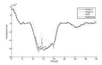
Fig. 5. Results from the two fusion approaches (solid black and gray lines) and the OLR (dotted line), showing the curvature estimate  $\hat{c}_0$ . As can be seen the curvature estimation can be improved by taking the other vehicles (gray line) and the host vehicle's driven curvature in account (solid black line). The dashed line is the reference curvature.
