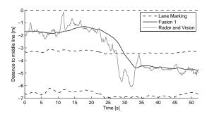
Illustration of the lateral movement over time of the leading vehicle  $l_{Tn}$  driving on a highway with three lanes, where the leading vehicle changes lane. The estimate from our fusion approach is given by the solid black lines and the raw measurement signal is shown by the solid gray line. The dashed lines shows the lane markings. In this example the distance to the leading vehicle is 65 m, see Fig. 7.
