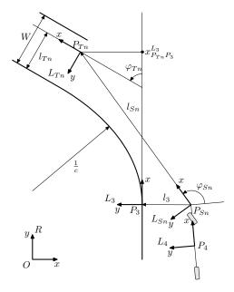
Relations between the leading vehicles Tn, the host vehicle and the road. The distance between the host vehicle path and the white lane to its left (where the road curvature is defined) is  $l_3$ . The lane width is W.
