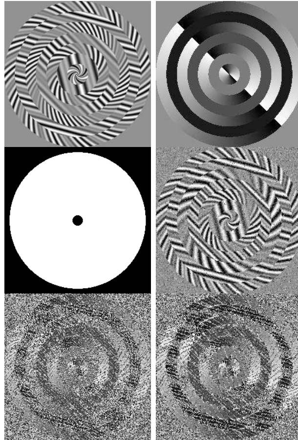
Fig. 14. Upper left: one instance of the test pattern. Upper right: ground truth orientation, encoded in gray levels. Middle left: index where the estimate and the ground truth are compared. Middle right: one instance of a test pattern with 1% Salt & Pepper noise and Gaussian noise of variance 0.01. Bottom left: raw orientation estimate from the gradient of the noisy image. Bottom right: raw orientation estimate from the Riesz transform of the noisy image.
