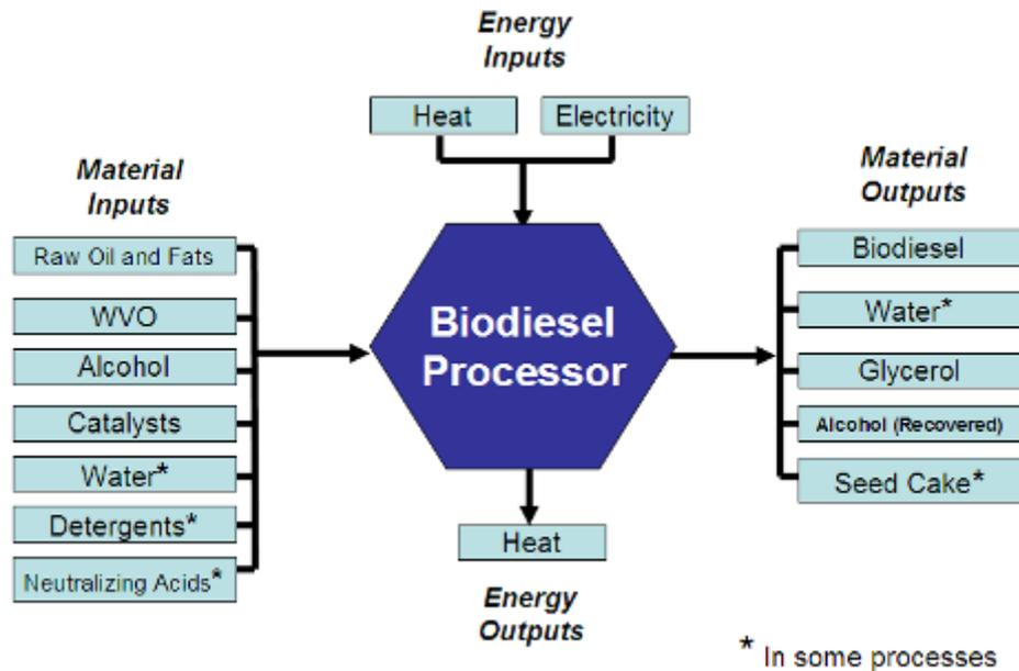
Figure 2: Biodiesel Production Diagram
