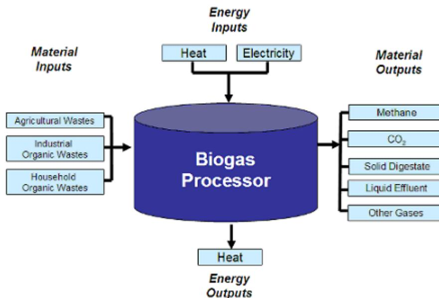
**Figure 1: Biogas Production**
