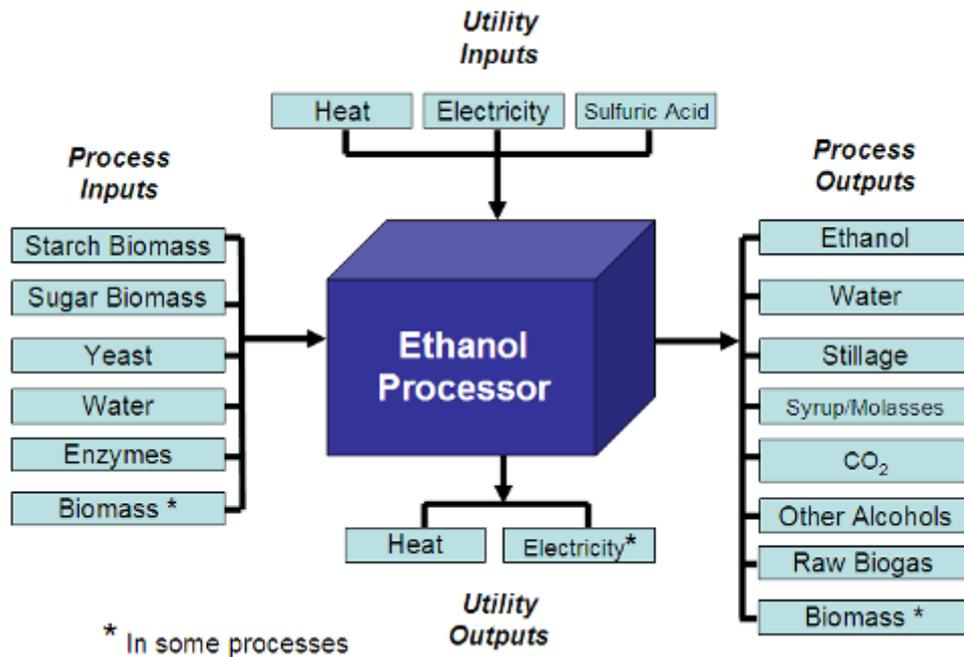
Figure 3: Ethanol Production Diagram
