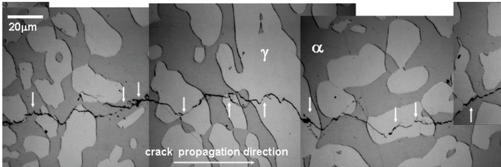
Fig. 2 Fatigue crack path in SAF 2507 bar material from a conventional fatigue propagation test. The arrows indicate where a crack branching appears.  $\gamma$  is the austenitic phase and  $\alpha$  is the ferritic phase.
