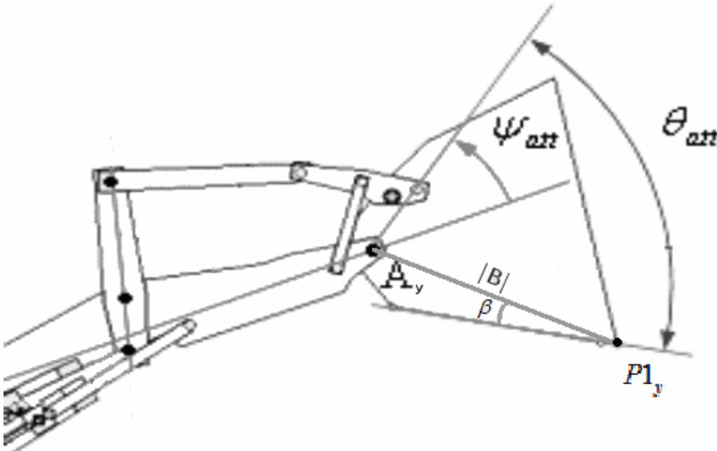
Figure 21, Calculation of height of bucket tip
