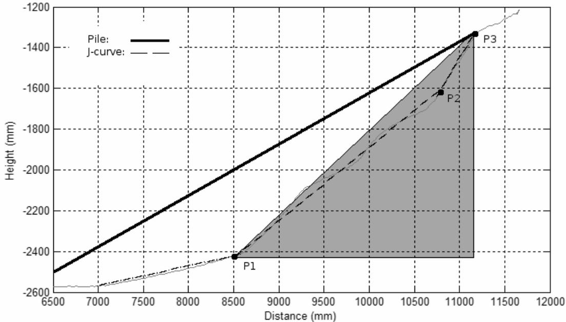
**Figure 23, Allowed placement of P2 (shaded area)**
