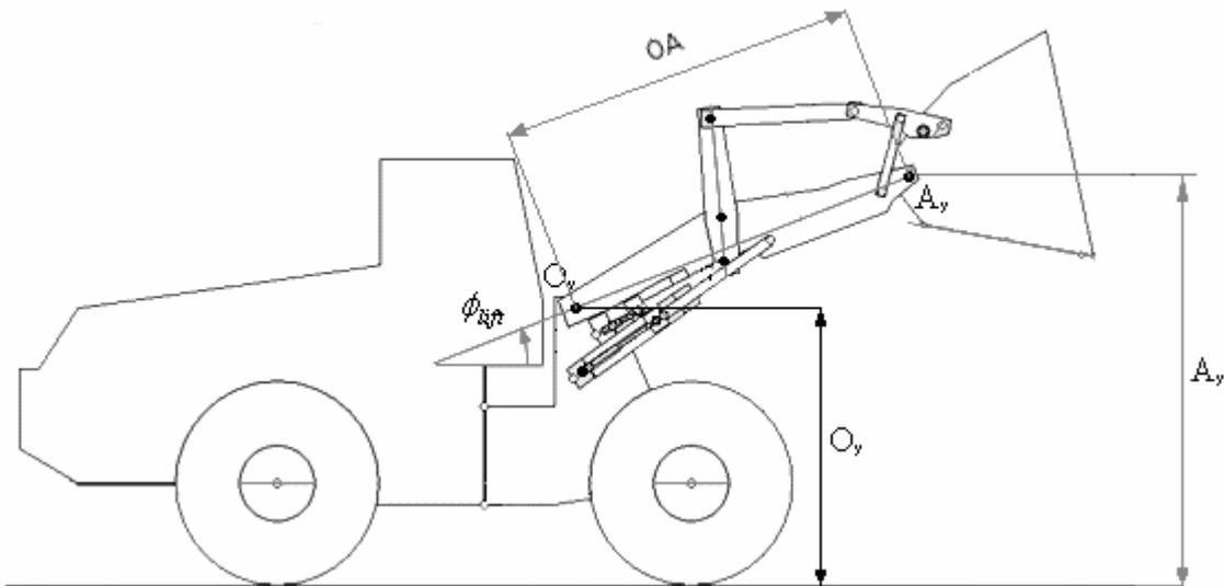
Figure 20, Calculation of height of A
