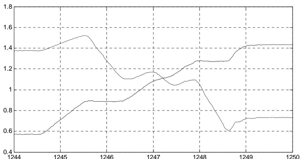
**Figure 17, The lift (increasing trend) and tilt (decreasing trend) collision**
