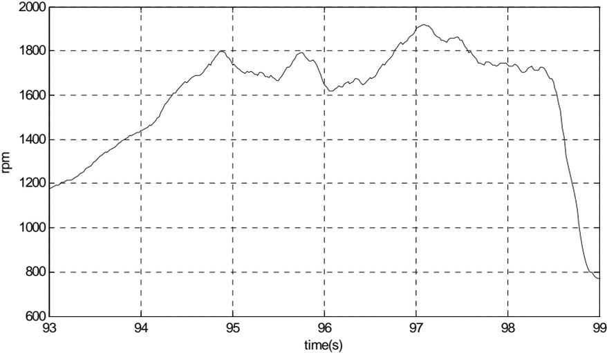
**Figure 35, Simple chic-chic engine RPM**
