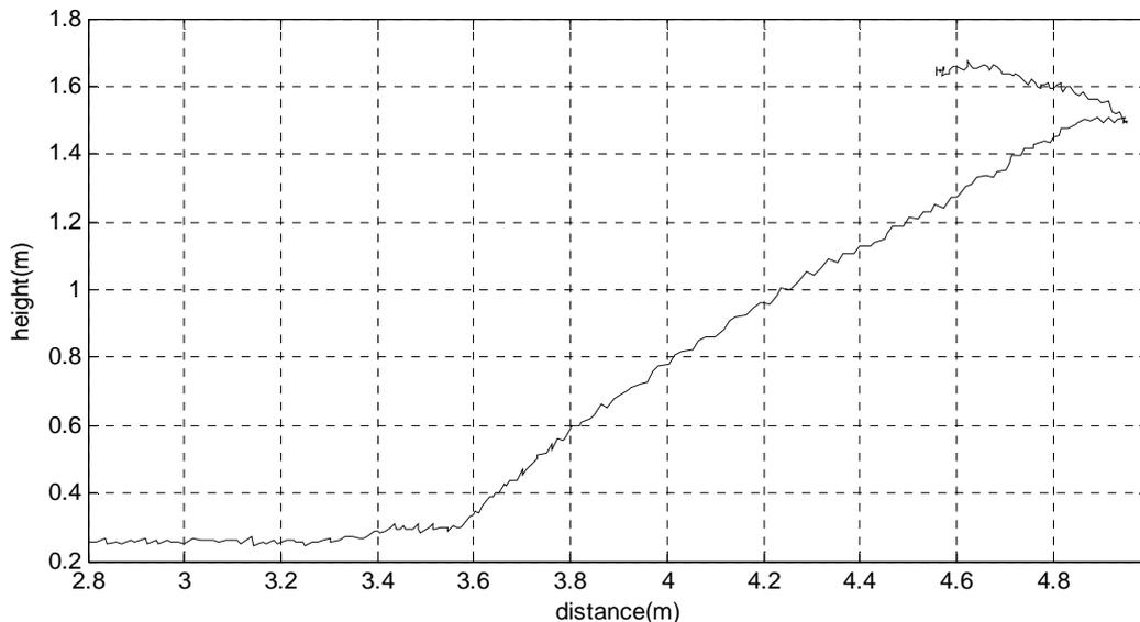
**Figure 32, J-curve test bucket tip movement**
