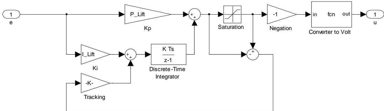
Figure 5, Example of PI-regulator with saturation compensation
