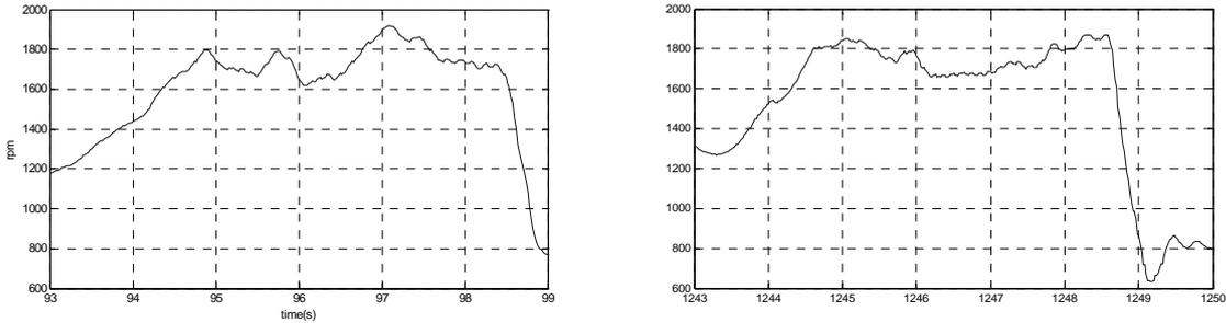
**Figure 37, Autonomous machine RPM (left) VS. Human driver RPM (right)**
