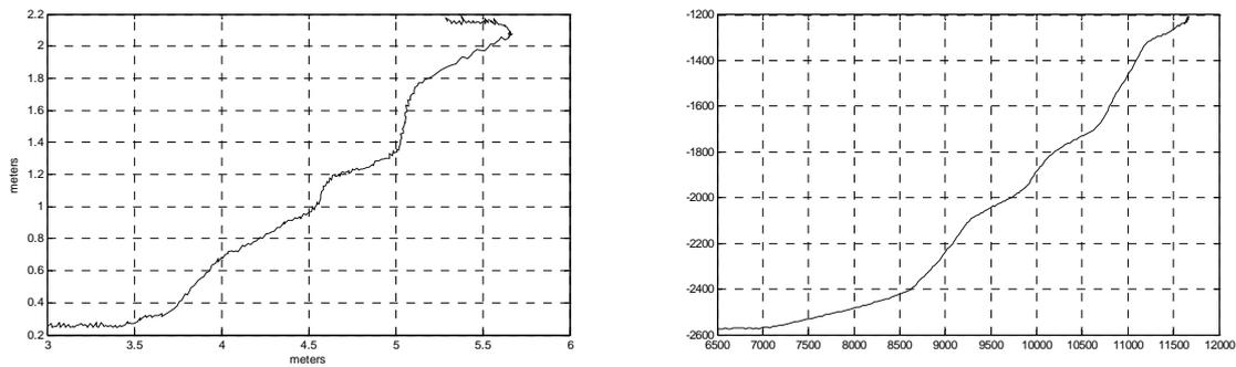
**Figure 38, Autonomous machine bucket tip movement (left) VS. Human driver bucket tip movement (right)**
