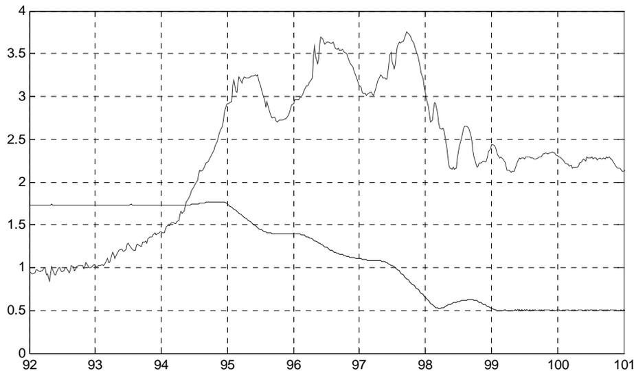
**Figure 16, Lift pressure (noisy) and tilt angle (smooth)**
