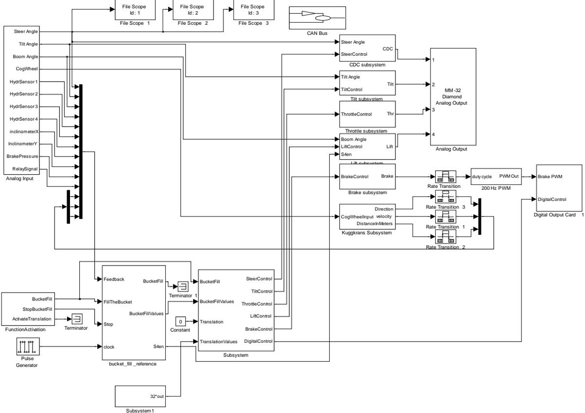
Figure 27, New Simulink main structure
