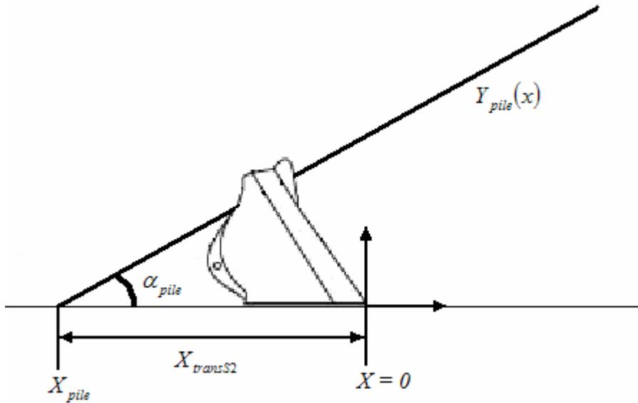
Figure 22, Pile profile calculation
