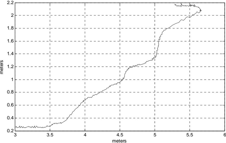
**Figure 36, Simple chic-chic bucket tip movement**
