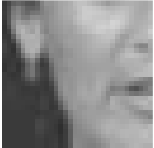
Fig. 10. Part of frame 28 of Miss America with losses and after error concealment by means of GMM. The square marks the place of a lost 8 \times 8 -block in the current frame. An estimation error is visible in the square.
