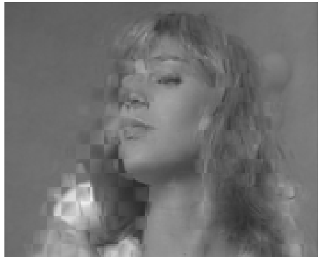
Fig. 6. Frame 51 of Suzie with losses and after error concealment by means of LMMSE.
