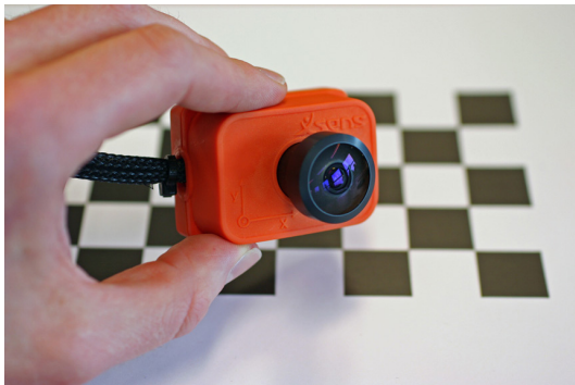
Figure 1: The sensor unit, consisting of an IMU and a camera. In this photo a fisheye lens was attached to the camera. The camera calibration pattern is visible in the background.
