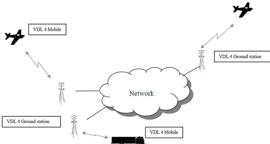
**Figure 16 General Overview of the VDL4 Communication system**
