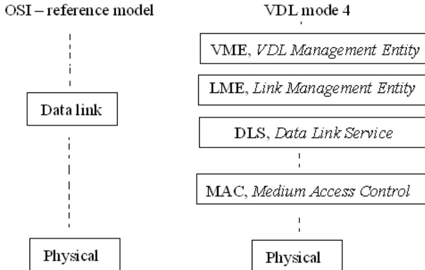
Figure 19 VDL4 referred to OSI-model
