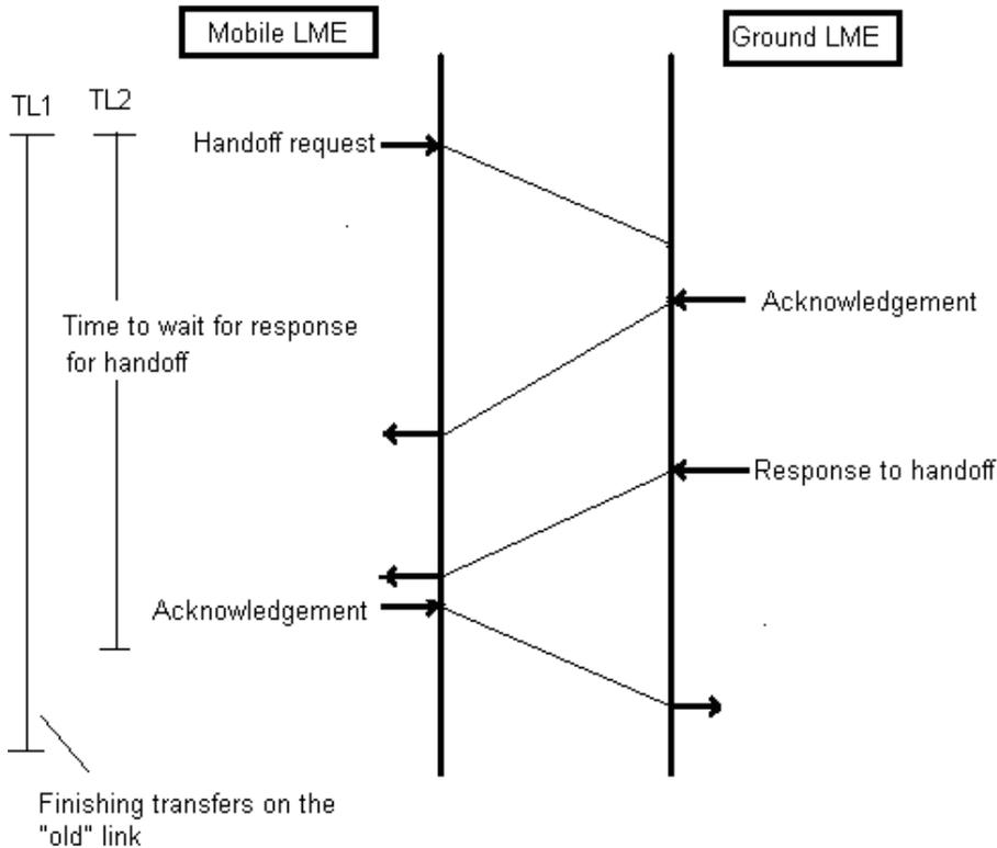
**Figure 21 Procedure for communication during mobile initiated handoff**
