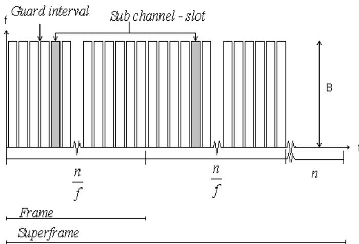
Figure 11 Illustration of TDMA
