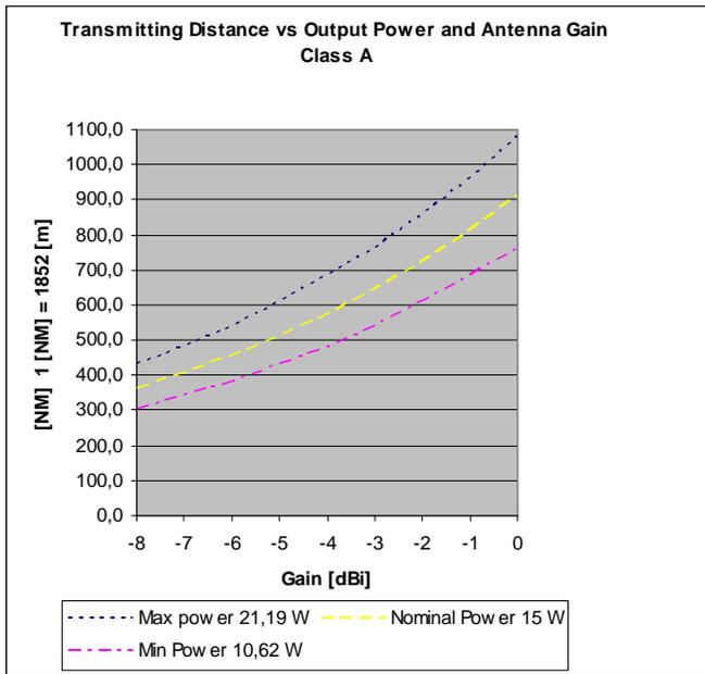
Figure 23 theoretical transmitting distance, class A transponder
