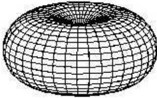
**Figure 7 Dipole omni-directional antenna pattern<sup>24</sup>**
