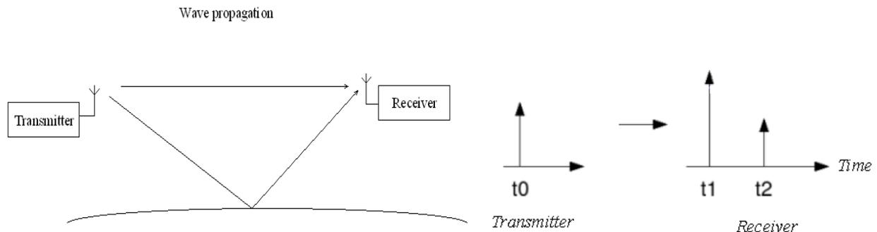
**Figure 4 Multipath in wireless communication**
