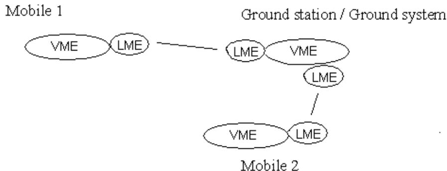
**Figure 20 The active functions in a point-to-point scenario in VDL4**
