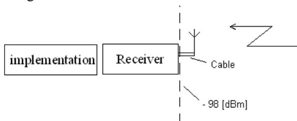
Figure 22 location of specified receiver sensitivity
