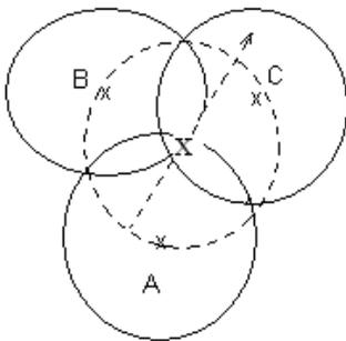
**Figure 30 Handoff decision based on duration of the point-to-point link and path of flight**
