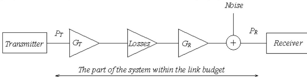
**Figure 6 Link budget in a wireless system**
