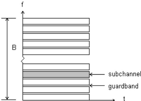
Figure 10 Illustration of FDMA
