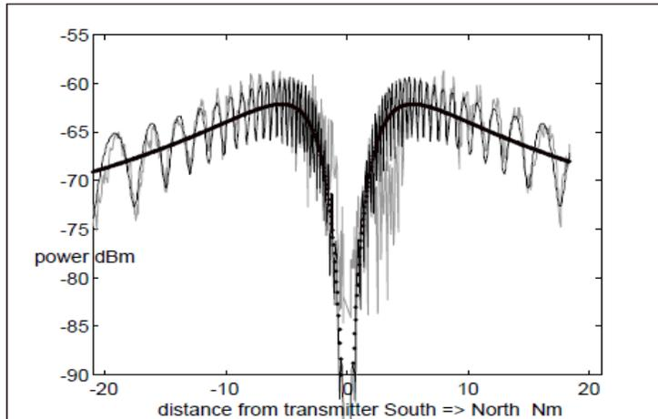
Figure 7 Power measurements and predictions for in flight receiver at FL200
