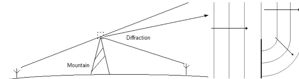
**Figure 5 Knife edge diffraction**
