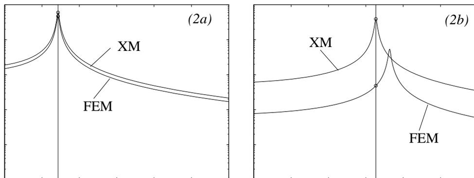
Figure 2. (2a) Transfer function contribution from the  $j$ th pair of modes of the FEM and XM. (2b) Transfer function contribution from the  $k$ th pair of modes. Both pair of curves should agree for well correlated FEM and XM. Circles and vertical lines indicate the XM resonance frequencies at which the functions are evaluated.
