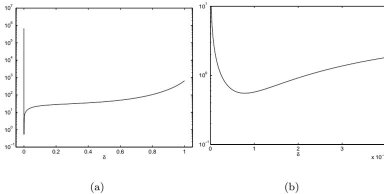
Figure 2: The mean square errors of the impulse response estimators for different values of  $\delta$ . ((b) is a zoomed part of the lower left corner of (a)).
