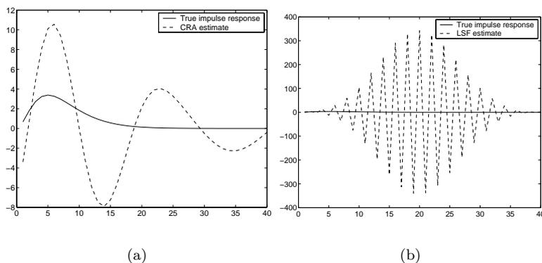
Figure 1: The (a) CRA and (b) least squares impulse response estimates compared with the true impulse response. (Notice that the scalings for the vertical axes are quite different).
