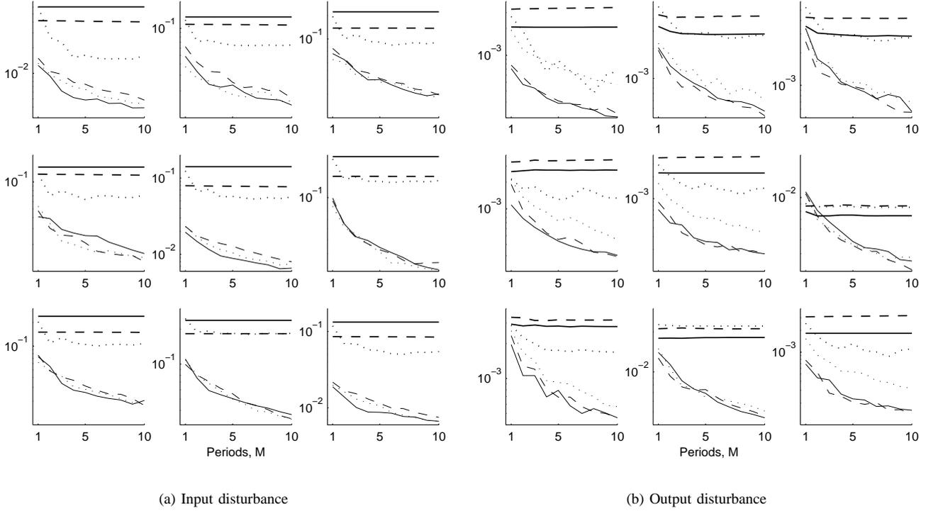
Fig. 4. Mean relative absolute error for different number of periods,  $M$ . A comparison between periodic (thick lines) and Gaussian (thin lines) disturbances using three different reference signals; multisine (solid), chirp with phase  $\phi = 0$  (dotted), and chirp with phase  $\phi = 1.89$  rad (dashed).
