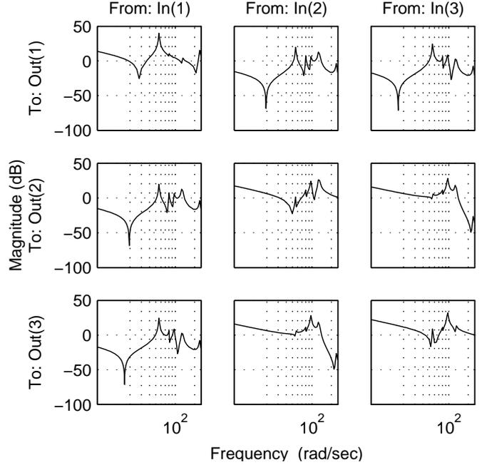
Fig. 2. Bode diagram of the transfer function from motor torque to motor speed.
