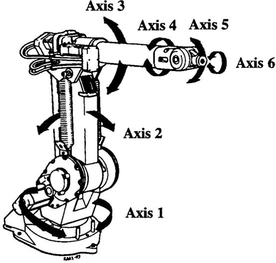
Fig. 1. The ABB manipulator IRB 1400.
