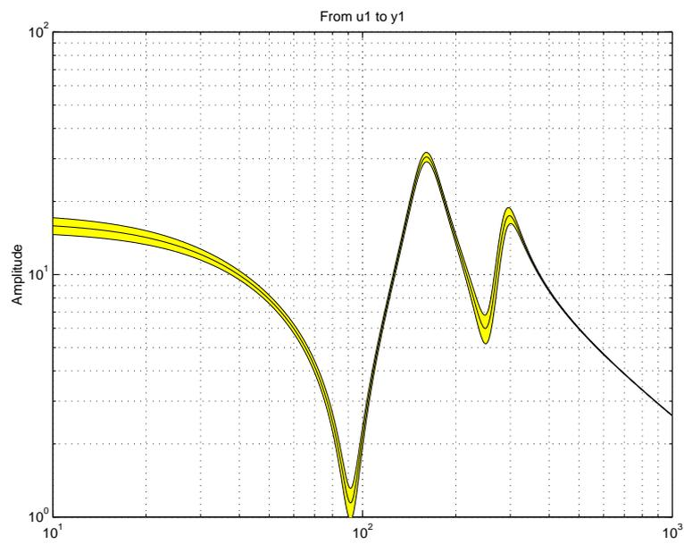
Fig. 6. Amplitude curve and confidence region for the mode obtained using Set2.
