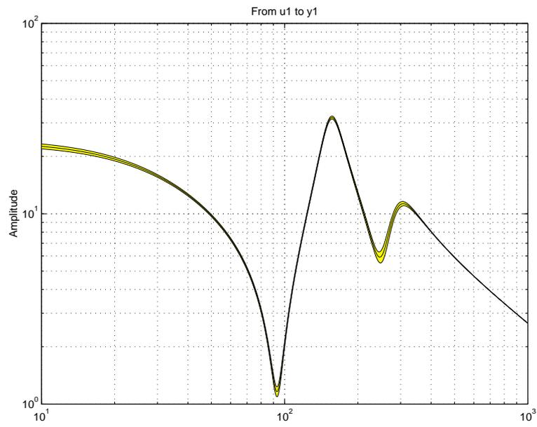
Fig. 5. Amplitude curve and confidence region for the mode obtained using Set1.
