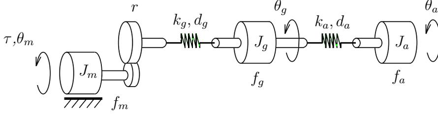
Fig. 2. Three-mass flexible model.
