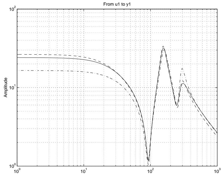
Fig. 3. Amplitude curves of physically parameterized models when  $K = 0$ . Solid – Set 1, Dashed – Set 3, Dash-dotted – Set 2.
