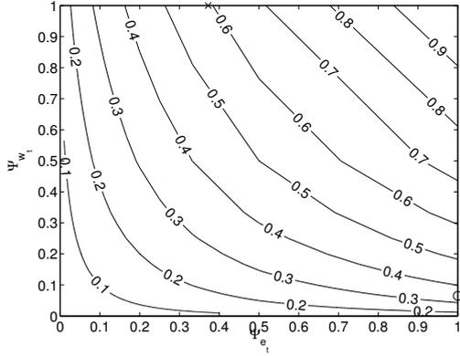
Fig. 5. Optimal filter performance,  $\bar{\kappa}_{(1,1)}(\Psi_{w_t}, \Psi_{e_t}) / \bar{\kappa}_{(1,1)}(1, 1)$  as a function of  $\Psi_{w_t}$  and  $\Psi_{e_t}$ . ( $\times$  denotes the noise in the first example and  $\circ$  the noise in the second example.)
