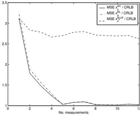
Fig. 6. Comparison of the ratios between MSE and CRLB for the different estimation schemes. (1000 Monte Carlo simulations.)
