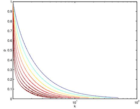
Fig. 4. The CRLB for the outlier situation. (Levels: [0.99, 0.98, 0.97, 0.95, 0.92, 0.87, 0.78, 0.64, 0.40 0], 0 being the uppermost level.) As a comparison, the BLUE yields unit variance for the estimator.
