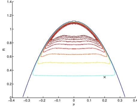
Fig. 3. The CRLB for the bi-Gaussian mixture distribution in (26). (Levels: [0.99, 0.98, 0.97, 0.95, 0.92, 0.87, 0.78, 0.64, 0.40 0], 0 being the outermost level.) Note that a Gaussian approximation yields unit variance. (× denotes the distribution simulated in Sec. 5.)
