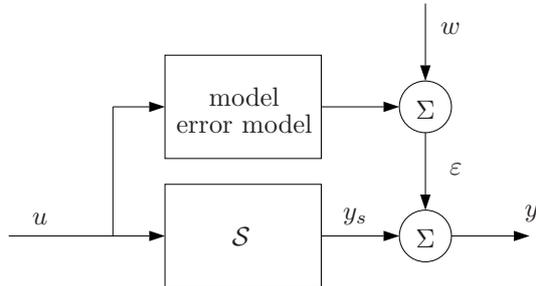
**Figure 1:** Block diagram of the model error model.
