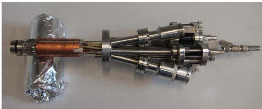
**Figure 3.2** Photo of the PVD source, an EFM3 UHV e-beam evaporator from Omicron®.
