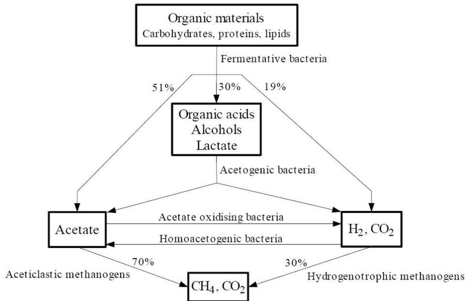
Figure 1. Carbon cycle for the biogas process. Modified after Kanokwan 2006.
