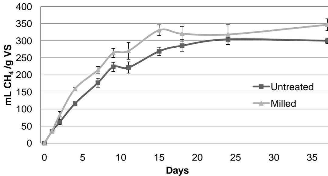
Figure 7. Mean methane production ( $n=3$ ) for untreated and milled *T. latifolia* in BD1 over 37 days. Error bars show standard deviation.
