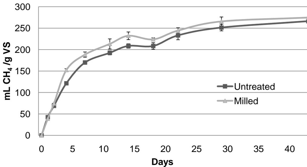
Figure 8. Mean methane production ( $n=3$ ) for untreated and milled *T. latifolia* in BD4 over 44 days. Error bars show standard deviation.
