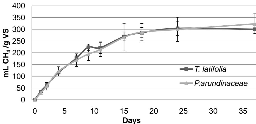
Figure 5. Mean methane production ( $n=3$ ) for *T.latifolia* and *P.arundinacea* in BD1 (Batch digestion 1) over 37 days. Error bars show standard deviation.
