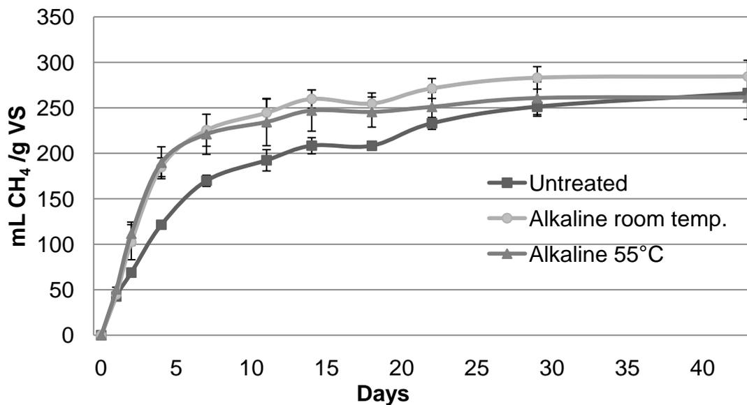
Figure 9. Mean methane production ( $n=3$ ) for untreated and alkaline pretreatment in BD4. Alkaline pretreatment at room temp. and 55 °C; both incubated with lime for 24 h. Error bars show standard deviation.
