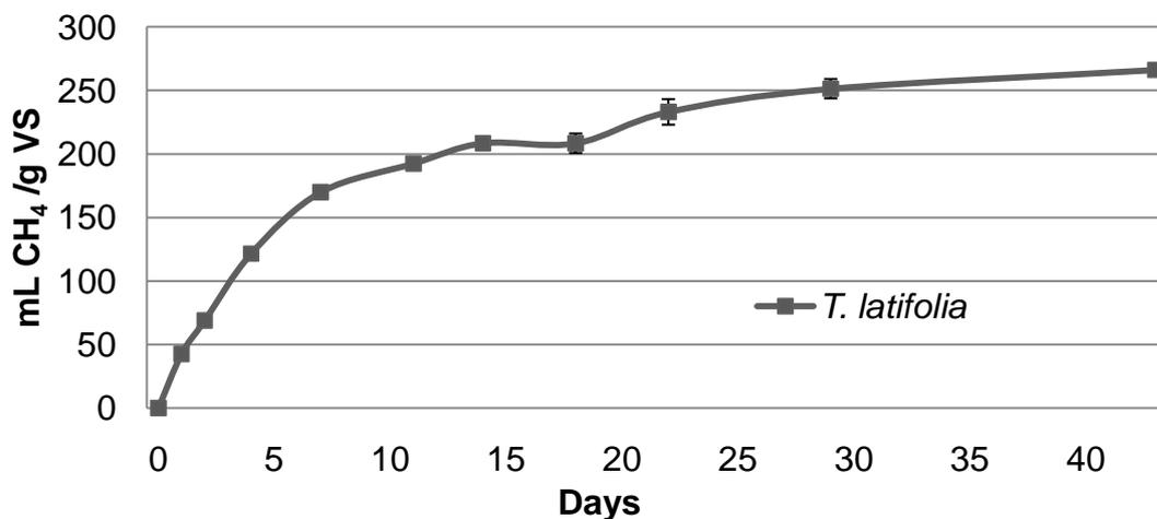
Figure 6. Mean methane production ( $n=3$ ) for *T.latifolia* in BD4 over 44 days. Error bars show standard deviation.
