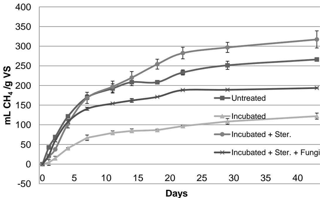
Figure 10. Mean methane production ( $n=3$ ) for untreated and incubated pretreatments in fungal experiment at BD4 over 44 days. Untreated has not been incubated as the others ( $30^{\circ}\text{C}$  for 46 days). Two of the incubated treatments has been sterilized and one of them also applied with white rot fungi. Error bars show standard deviation.
