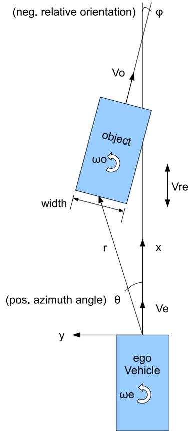
Figure 2.2: Overview of how the states and some of the input signals are defined.
