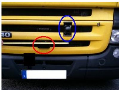
Figure 4.1: The placement of the laser (red) and the radar (blue) on the truck.
