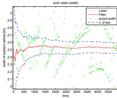
Figure 4.9: The width of the tracked vehicle from observations and filter together with the actual width.
