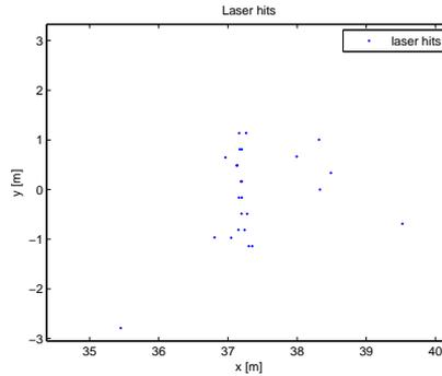
Figure 3.6: Laser hits before filtering.
