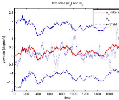
Figure 4.8: Yaw rate of tracked vehicle (filter) and ego vehicle (ego data).
