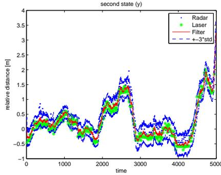
Figure 4.5: Relative distance in lateral direction from observations and filter.
