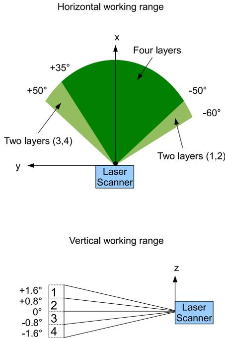
Figure 4.2: The working range of the laser scanner.
