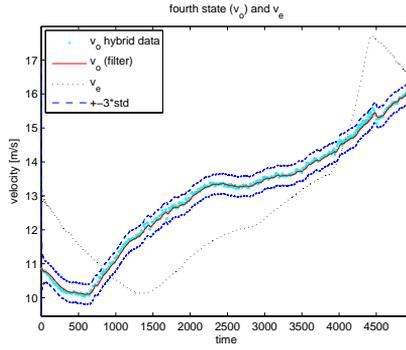
Figure 4.7: Velocity of tracked vehicle from "hybrid data" and filter.
