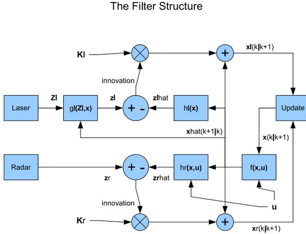
Figure 2.1: Overview of the structure of the filter.
