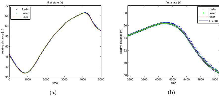
Figure 4.4: Relative distance in longitudinal direction from observations and filter.
