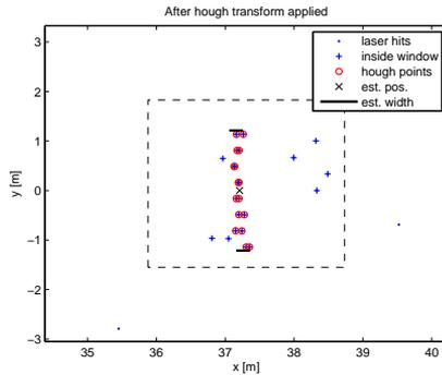
Figure 3.8: After hough transform applied on laser hits inside window.
