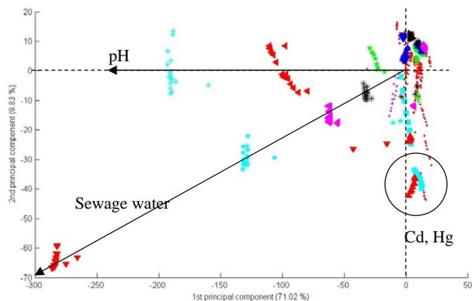
Fig. 3: Data from laboratory measurements showing, in the first two principal components of a PCA plot, that different types of substances in the drinking water may give rise to deviations in different directions of the PCA plot. There are four different concentrations of sewage water along the "sewage water axis" and two different pH values along the "pH axis".
