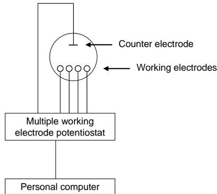
Fig. 2. Schematic illustration of the electronic tongue measurement setup. The sensing probe contains four working electrodes and a counter electrode. A "multiple working electrode potentiostat" and a personal computer are used to supply voltage pulses and to measure the corresponding current transients.
