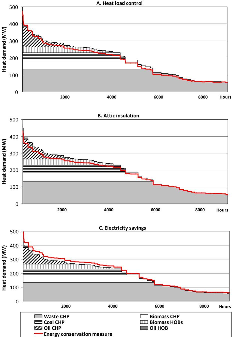
Figure 7.2. Annual DH demand including the DH plant operations in Linköping, where the red line represents the effect the ECM has on the DH demand. A. represents the measure Heat load control; B. Attic insulation and C. Electricity savings.
