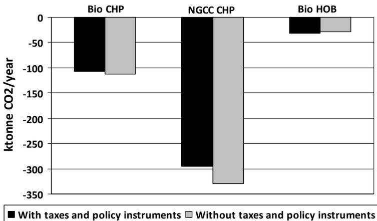
Figure 7.4. Difference in annual global CO<sub>2</sub> emissions (ktonne/year) compared to the reference case for the different technologies, when the taxes and policy instruments are included or excluded (tradable CO<sub>2</sub> emission permits are included in both scenarios).
