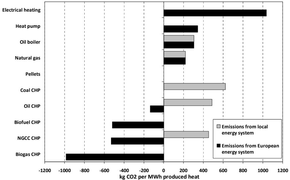
Figure 4.3. Net global CO<sub>2</sub> emissions per MWh produced heat (red bars) for different fuels and technical solutions when coal condensing power is marginal electricity production in the European electricity system (Werner, 2001; Werner and Karlsson, 2010).
