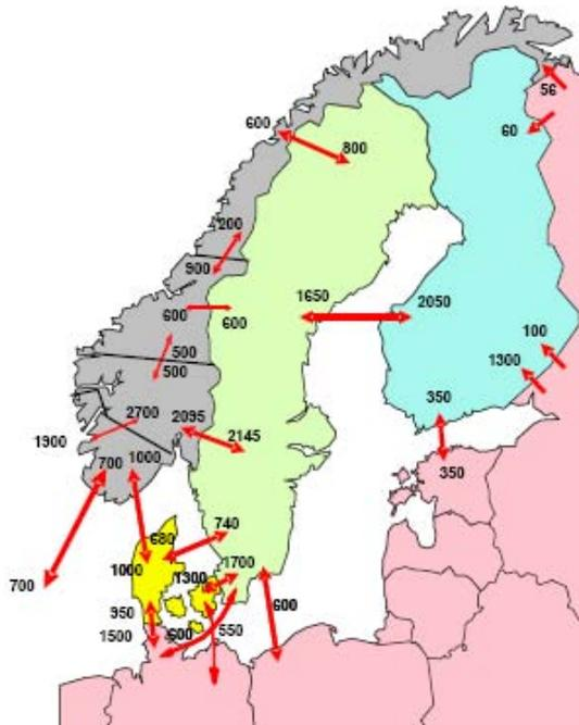
Figure 3.2. Power transmission capacities, in MW (Nord Pool, 2010b).
