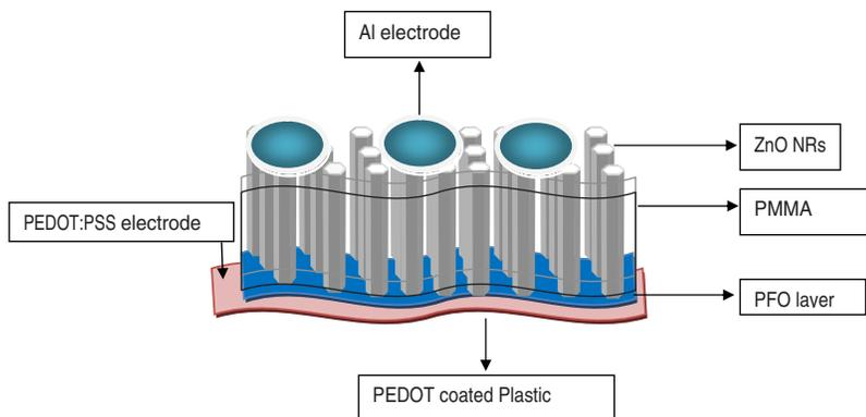
FIG. 1. (Color online) Schematic illustration of ZnO NRs/PFO hybrid device on PEDOT:PSS coated flexible plastic.
