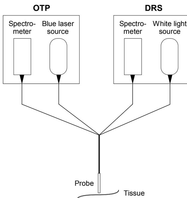
Figure 3.1 Hardware design of OTP [22] and diffuse reflection spectrometer [23]
