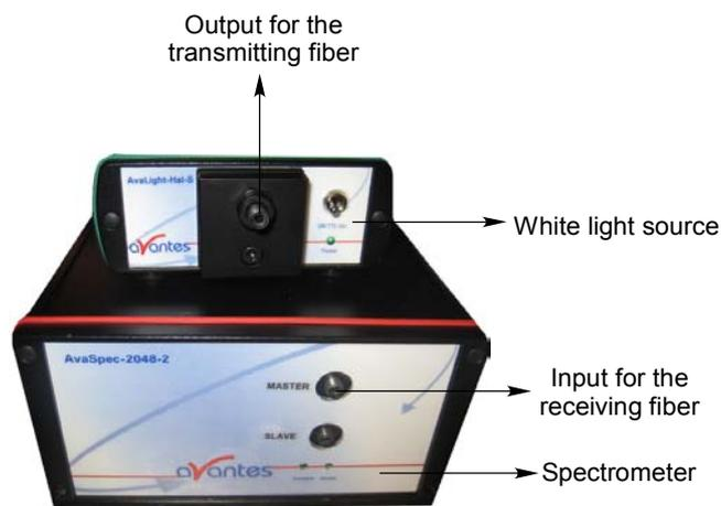
Figure 3.2 Devices for white light transmission and collection
