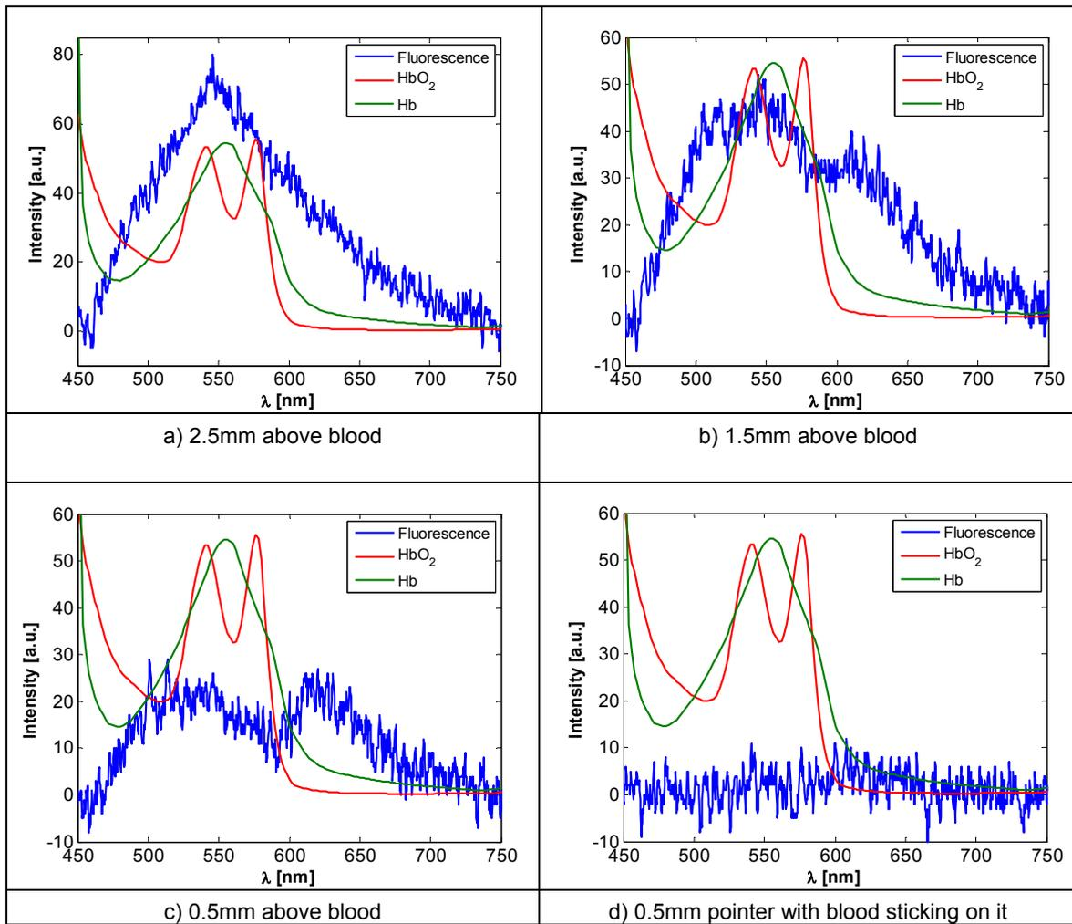
Figure 10.1 Blood and hemoglobin fluorescence spectra on standard C
