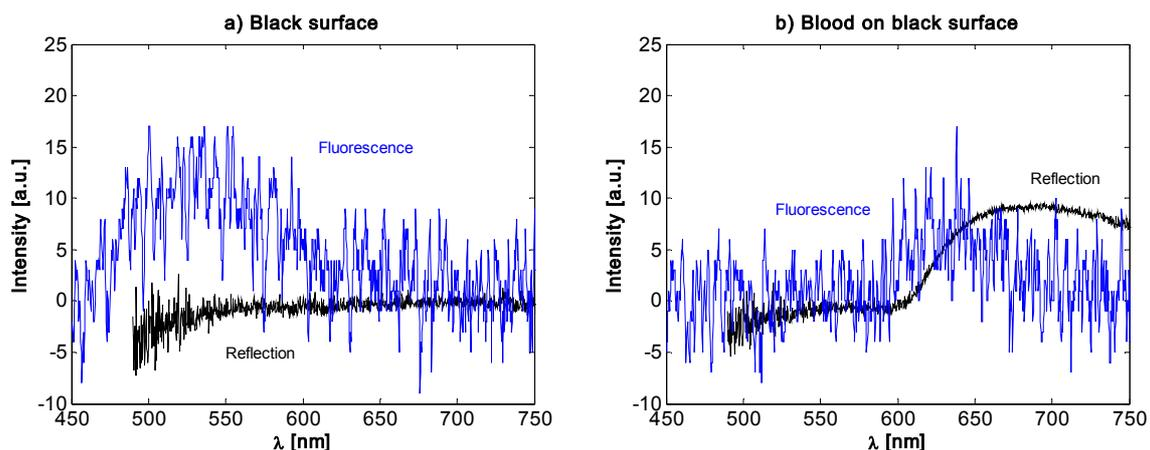
Figure 4.3 Autofluorescence of a black surface with and without blood
