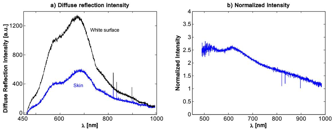
Figure 3.7 Example of a normalized skin diffuse reflection spectrum
