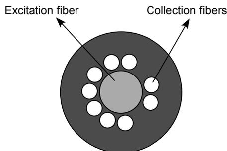
Figure 3.3 Optical fiber probe [22]
