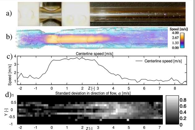
Fig. 1. a) An image of the phantom. b,c,d) Visualization of measurements at Re = 1000. b) A streamline visualization enclosed by an isosurface. c) A plot of the centerline speed. d) A SD map. Y and Z are dimensionless long measures that show the distance from the stenosis center.
