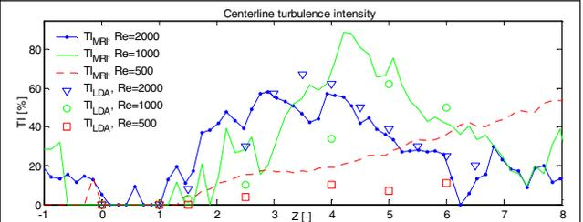
Fig. 2. Centerline TI for Re 500, 1000, 2000 in the flow-direction as measured with MRI and LDA. On the horizontal axis, the dimensionless long measure Z shows the distance from the stenosis center.
