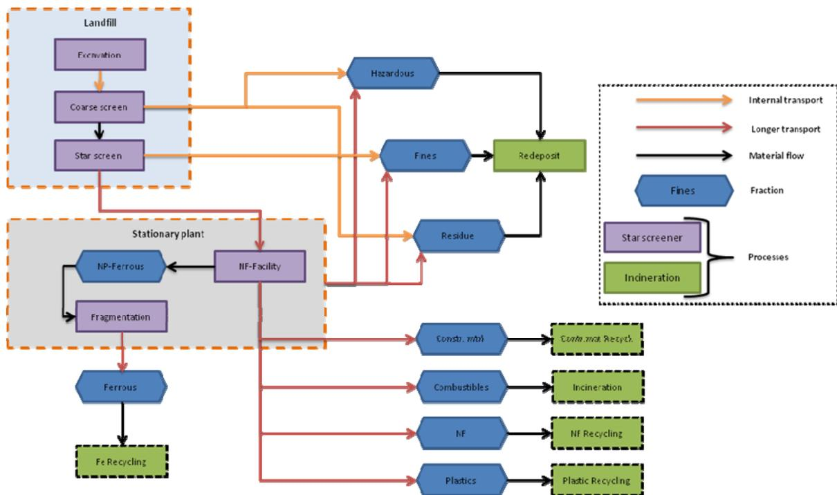
Figure 3. Process model over the stationary plant scenario
