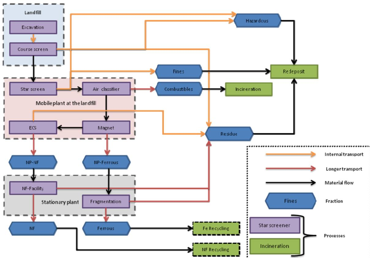
Figure 2. Process model over the mobile plant scenario
