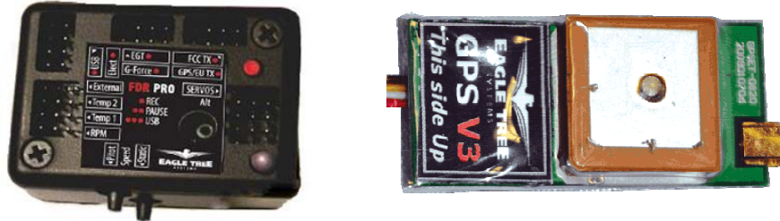
Figure 12. The USB flight data recorder (left) and GPS antenna (right) used as payload for the aircraft design.
