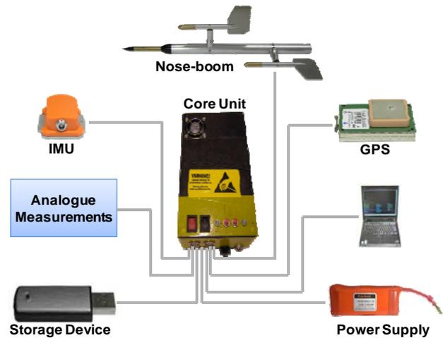
**Fig. 7 The flight test equipment**
