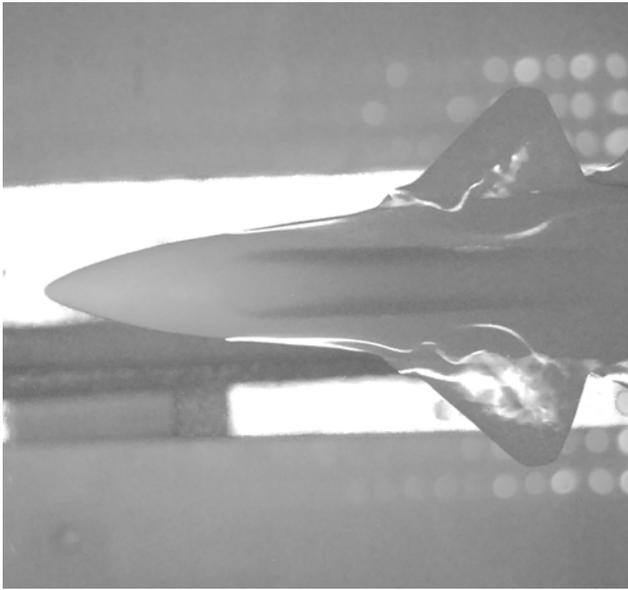
**Fig. 13 Interaction between forebody vortex and canard vortex**
