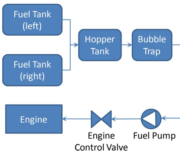
**Fig. 10 Scheme of the installed fuel system**
