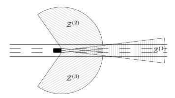
Figure 1: The observation spaces of the front looking radar is denoted  $\mathscr{Z}^{(1)}$  and the observation spaces of the side radars are  $\mathscr{Z}^{(2)}$ and  $\mathcal{Z}^{(3)}$ .
