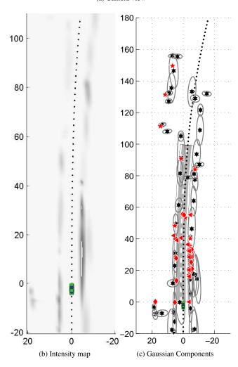
Figure 2: The image in Figure (a) shows the driver's view. The intensity map  $v_{k|k}$  is shown in Figure (b). The Gaussian mixture (mean and covariance ellipse) as well as the measurements from the radars are shown in Figure (c). The red stars are obtained by the front radar ( $\mathbf{Z} \in \mathscr{Z}^{(1)}$ ), the diamonds by the left radar ( $\mathbf{Z} \in \mathscr{Z}^{(2)}$ ) and the triangles are by the right radar ( $\mathbf{Z} \in \mathscr{Z}^{(3)}$ ).
