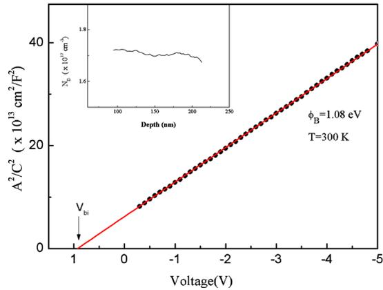
FIG. 1. (Color online) Typical  $C$ - $V$  measurements performed at 75 kHz to evidence Schottky behavior of the Au/GaN device from  $A^2/C^2$ - $V$  linear relationship. Inset witnesses homogeneous spatial distribution of free carrier.
