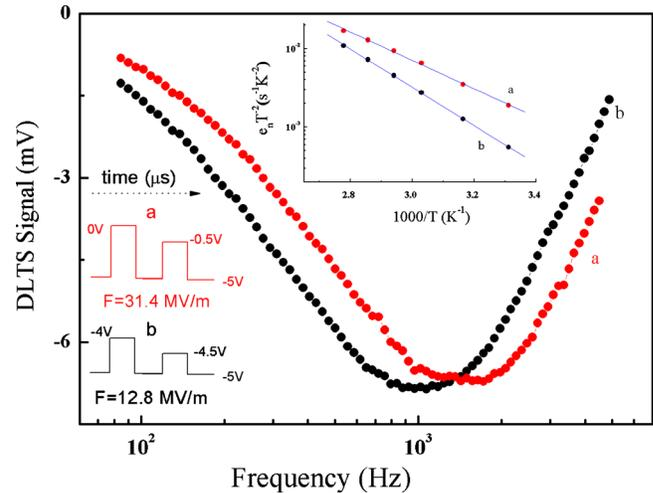
FIG. 2. (Color online) Representative frequency-DLTS spectra displaying the field enhanced emission signatures of an electron trap  $E$ . The applied excitation pulse conditions for DLTS scans (a), (b) are sketched in the respective colors of the curves, here pulse width,  $t_p = 20 \mu\text{s}$ . Inset demonstrates the associated Arrhenius plots at two representative fields.
