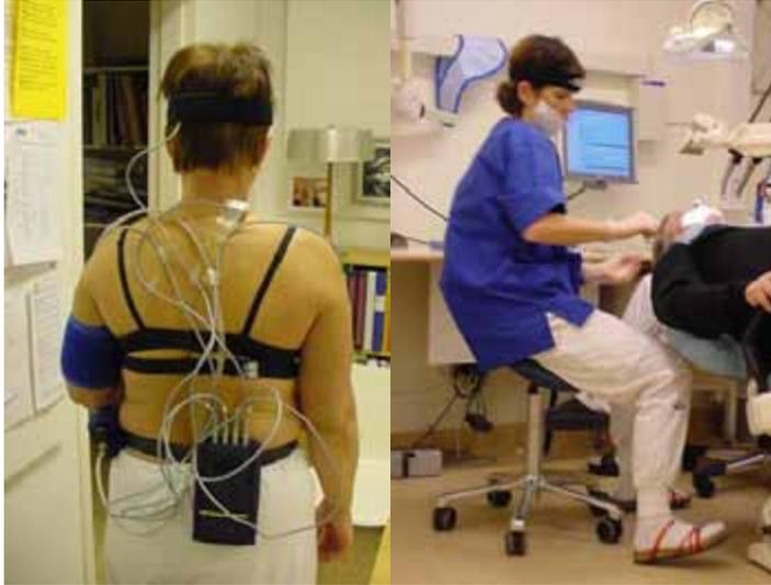
Figure 4. Inclinometer datalogger and inclinometers attached on a dentist.
