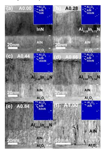
**Figure 1** (a)-(f) Cross-sectional TEM images showing the Aseries of the Al<sub>x</sub>In<sub>1-x</sub>N samples grown on AlN buffer layer and Al<sub>2</sub>O<sub>3</sub> substrate and corresponding selective area diffraction pattern for each sample along [11-20].
