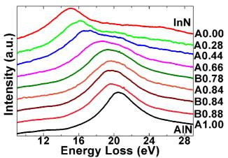
**Figure 2** Low-loss EEL spectra showing the shift in plasmon energy  $(E_p)$  of the A and B  $Al_xIn_{1-x}N$  samples in compositional order from InN (top spectrum, x=0) to AlN (bottom spectrum, x=1).
