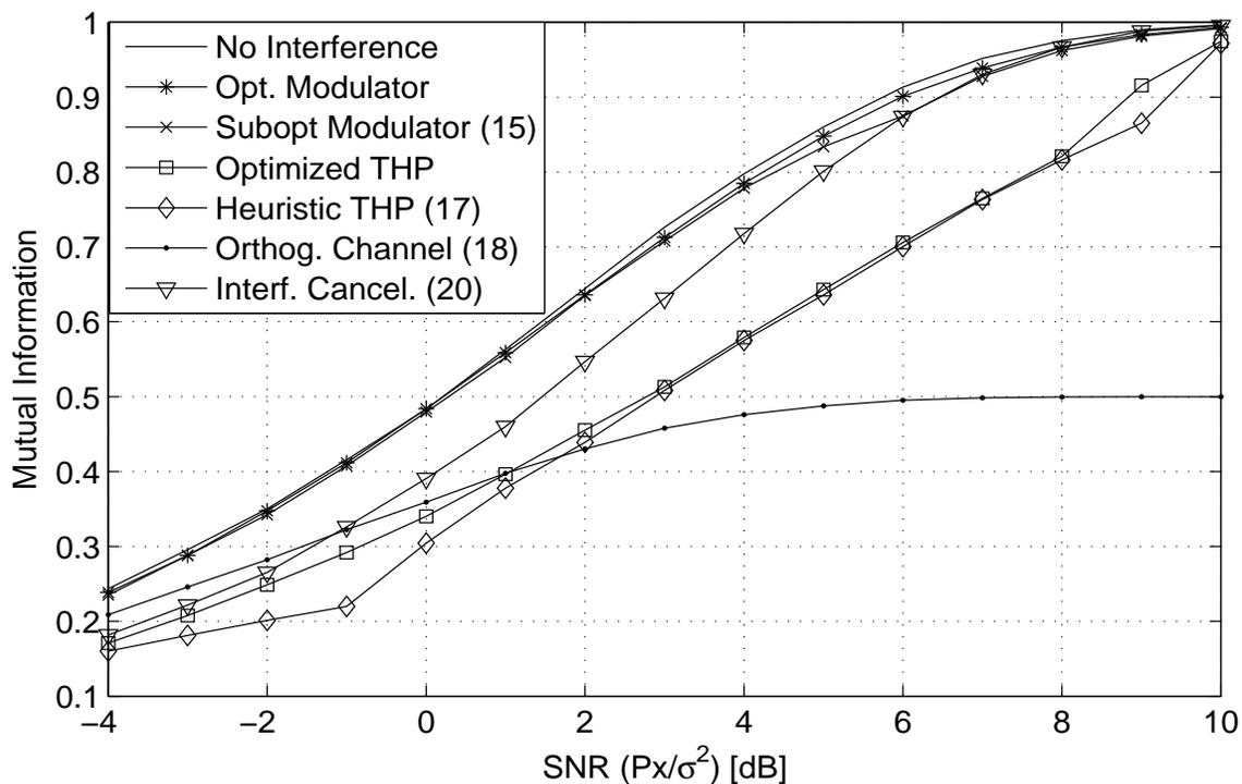
Fig. 2. Mutual information for binary signaling in binary interference, with  $\text{INR}(P_z/\sigma^2) = 6$  dB.
