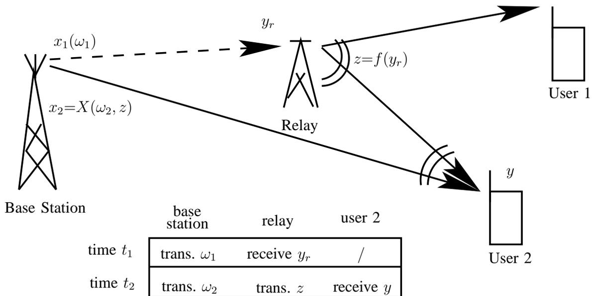
Fig. 1. The base station transmits  $\omega_1$  to user 1 during time slot  $t_1$  and  $\omega_2$  to user 2 during time slot  $t_2$ . The relaying signal  $z=f(y_r)$  dedicated for user 1 appears as “interference” for user 2. With non-causal knowledge of  $z$ , the base station can design a DPC modulator  $x_2 = X(\omega_2, z)$  given the information symbol  $\omega_2$  and the interference  $z$ .
