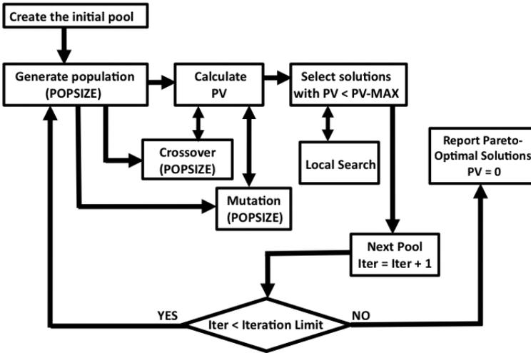
**Figure 4.3** Principle design in finding Pareto-optimal configurations.
