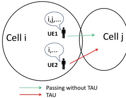
Figure 5.5 UEs holding different TALs in one cell.
