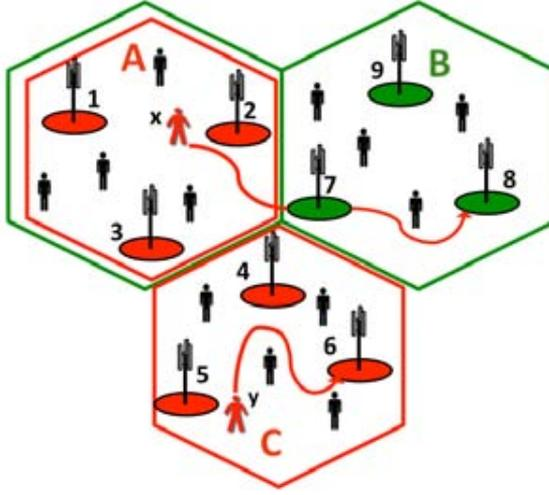
**Figure 6.3** An example of how to collect part of UE traces.
