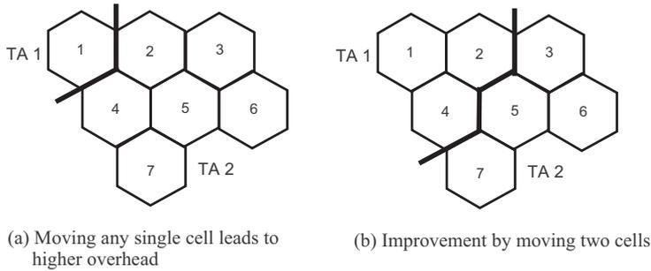
**Figure 3.1** An example of the dependency between cell moves.
