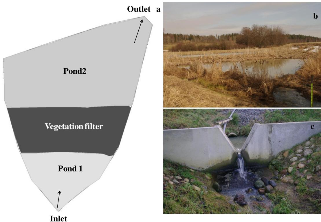
**Figure 2.** a) Schematic drawing of Skilleby wetland with the inlet, pond 1, vegetation filter, pond 2 and the outlet marked out. (Drawing by Anna Senior) b) Photo of the wetland, seen from the inlet. c) Photo of the v-notch at the inlet.
