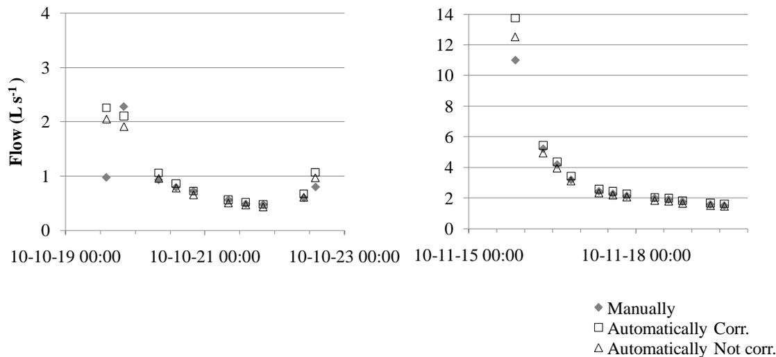
**Figure 10.** Automatically registered and manually measured flow values during the October (a) and November (b) sampling periods in Skilleby wetland in 2010. Manual flow measurements were done at the inlet v- notch, using stop watch and bucket. Automatically registered values are also shown, both uncorrected and corrected with a factor of 1.1.
