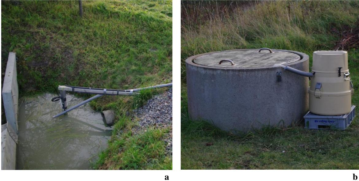
**Figure 3.** Skilleby wetland before the v- notch at the inlet with the sampling pipe visible (a), and the outlet well with the ISCO- sampler (b).
