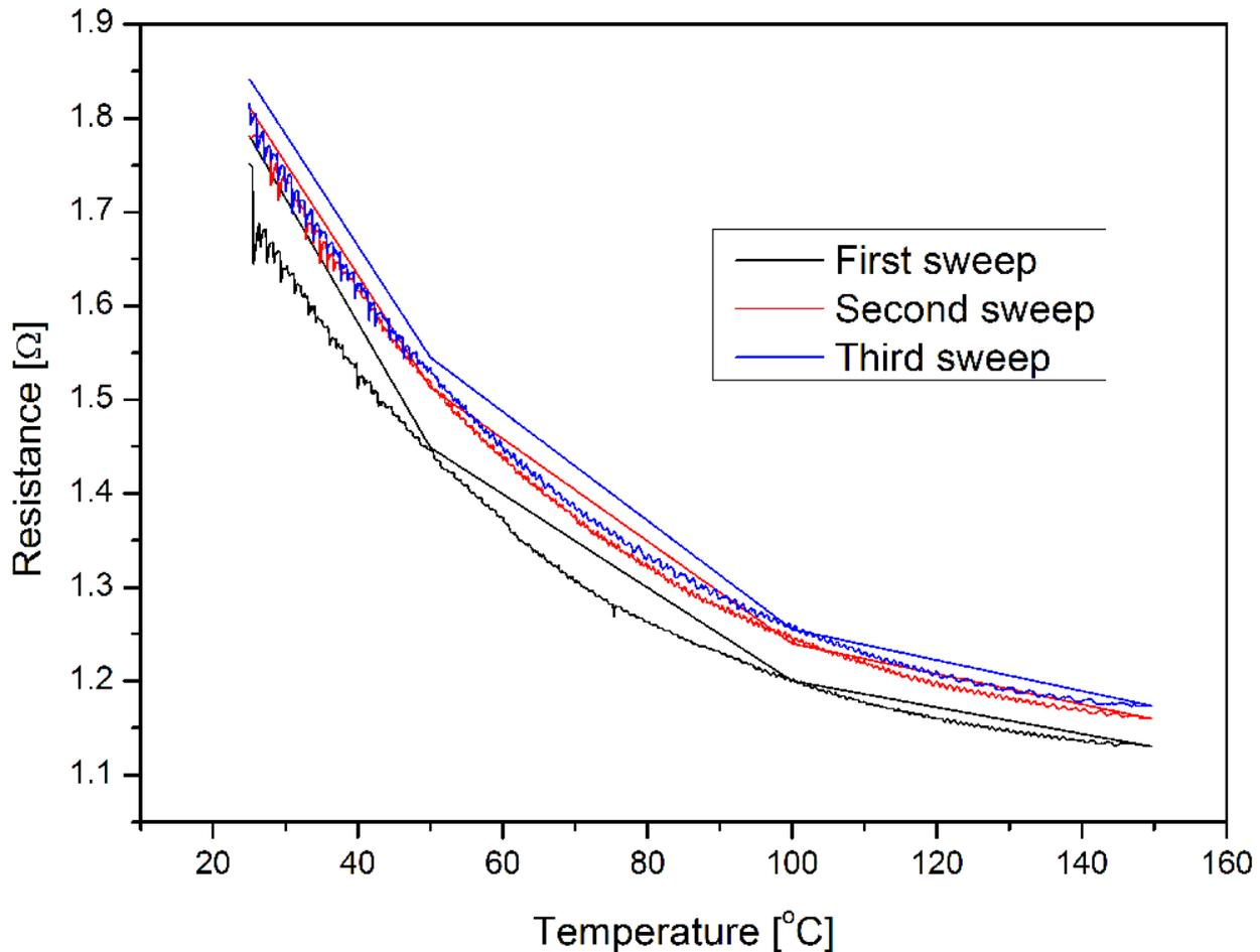
**Figure 2:** Plot showing change in resistance with temperature of the multi layer device. The heating rate was  $10\text{ }^{\circ}\text{C min}^{-1}$ . The resistance was then recorded on returning to 100, 50 and 25  $^{\circ}\text{C}$
