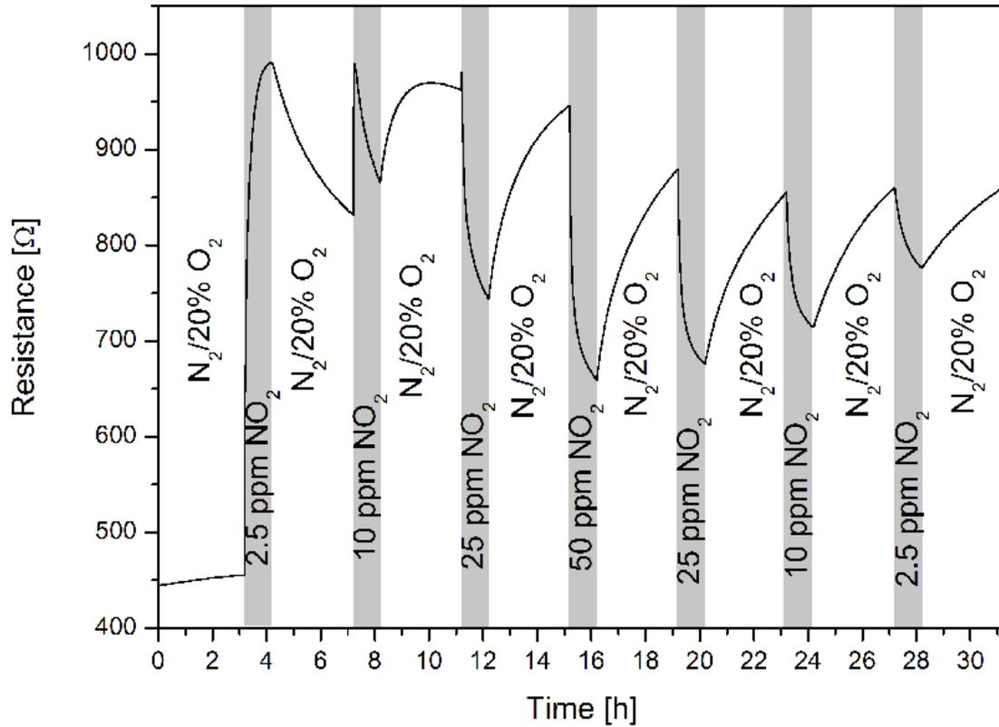
**Figure 4:** Response of single layer graphene sensor towards  $\text{NO}_2$  in a carrier gas of  $\text{N}_2$  with 20%  $\text{O}_2$  at 25 °C. Plot shows change in response direction during the first 10 ppm  $\text{NO}_2$  pulse.
