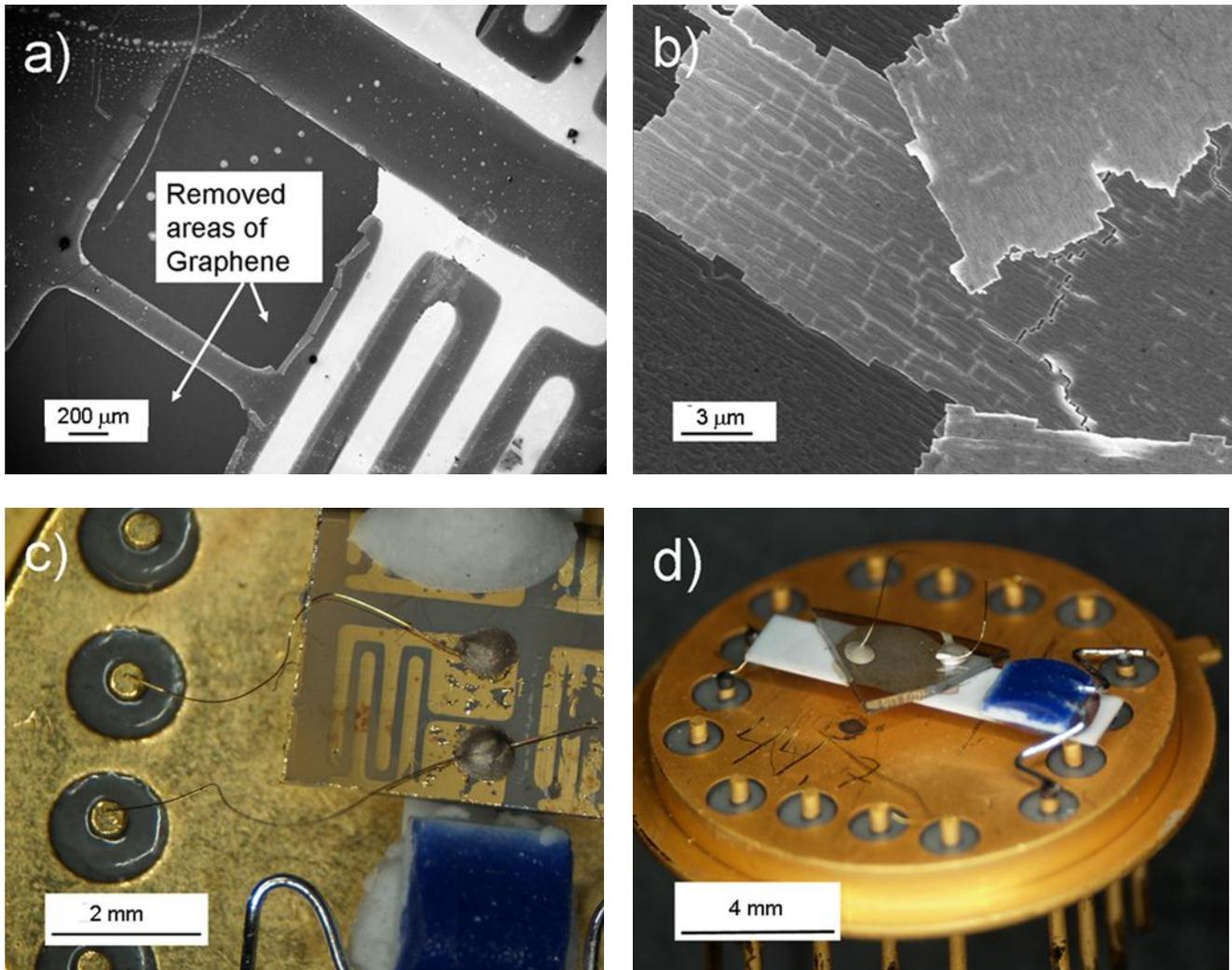
**Figure. 1:** SEM images showing; a) interdigitated finger electrode structure on multilayer graphene with bond pads and underlying graphene removed. b) SEM image showing flakes of multi layer graphene (light grey) at edge of removed bond pad showing SiC underneath (dark grey). The step edges of the SiC are just visible. c) wire bonded multi layer device on header showing heater and temperature monitor (blue). d) wire bonded single layer device.
