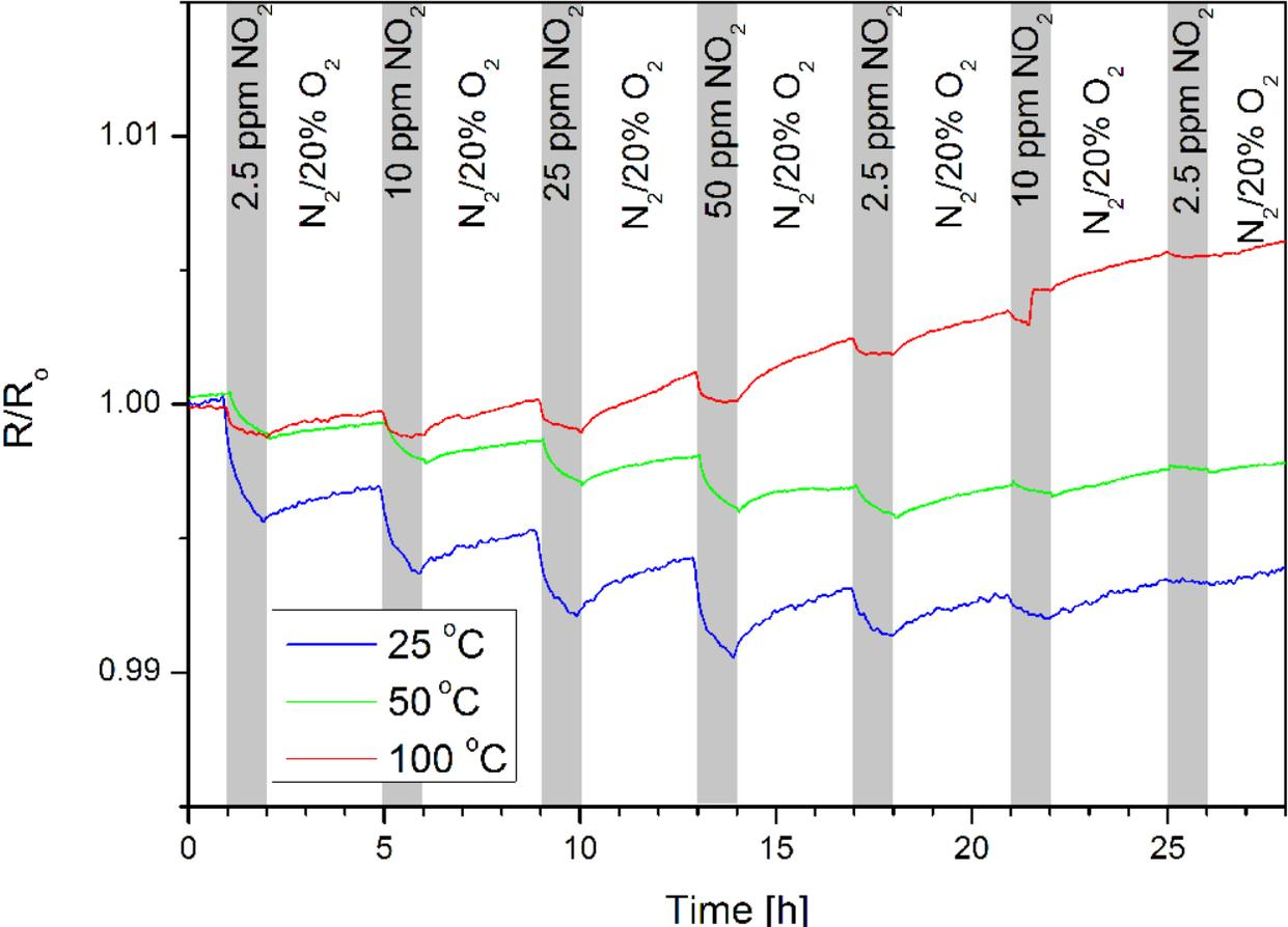
**Figure 3:** Response of multi layer graphene sensor towards NO<sub>2</sub> pulses at 25, 50 and 100 °C in a carrier gas of N<sub>2</sub> with 20% O<sub>2</sub>.
