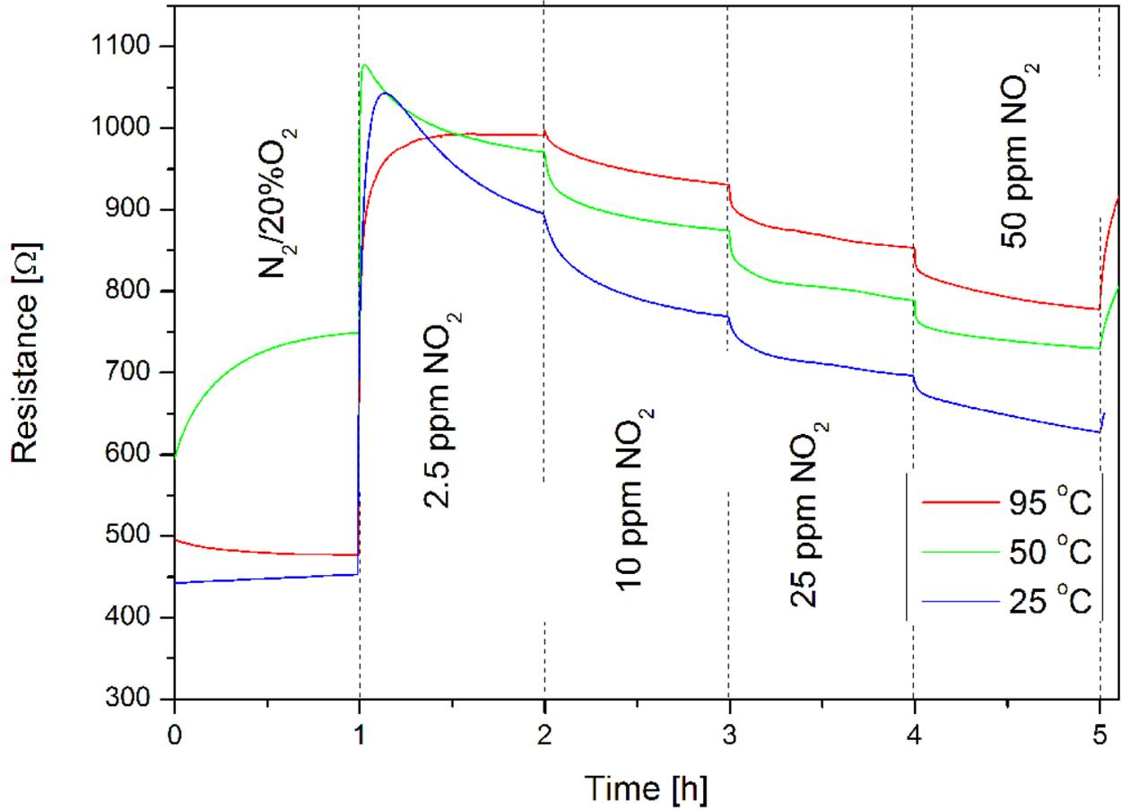
**Figure 5:** Response of single layer graphene sensor towards stepwise increases in NO<sub>2</sub> in a carrier gas of N<sub>2</sub> with 20% O<sub>2</sub>. Plot shows change in response direction with increasing NO<sub>2</sub> concentration.
