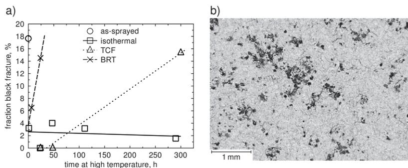
Fig. 3. Fraction of black fracture. a) Fraction black fracture measured by SEM EDS mapping. b) Specimen subjected to TCF 300 cycles, SEM backscatter electron image. Black fracture can be seen as dark areas which are exposed  $\text{Al}_2\text{O}_3$ .
