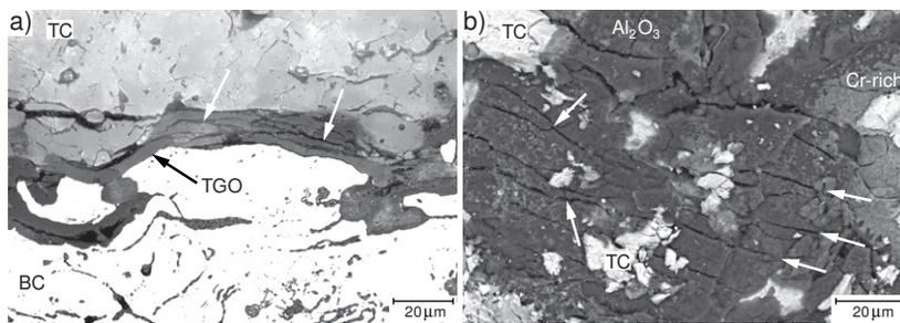
Fig. 5. Damaged interface TGO, marked by arrows, in specimen subjected to 300 cycles of TCF. a) Cross-section, light-optic micrograph. b) Fracture surface after adhesion test, SEM backscatter electron image.
