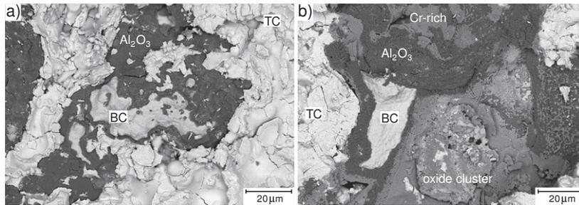
Fig. 4. Characteristics of black fracture, SEM backscatter electron images. a) BRT 1150 cycles. The TGO consists of a thin layer of relatively pure  $\text{Al}_2\text{O}_3$ , the image shows both TGO/TC and BC/TGO fracture. b) TCF 300 cycles. The image shows TGO/TC and BC/TGO fracture as well as a cut-through oxide cluster. Besides  $\text{Al}_2\text{O}_3$  and mixed–element oxide clusters, the TGO can be seen to contain colonies of Cr-rich oxides on top of the  $\text{Al}_2\text{O}_3$ .
