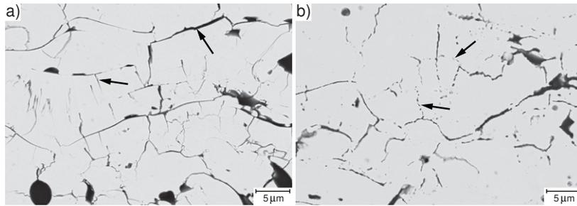
Fig. 1. Microcracks and delaminations in the top coat, SEM backscatter electron images. a) An as-sprayed specimen, arrows mark vertical through-splat microcracks and horizontal between-splat delaminations. b) Evidence of sintering in specimen subjected to 290 h of isothermal oxidation at 1100 °C, arrows mark sintered cracks.
