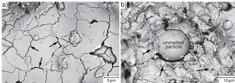
Fig. 2. Characteristics of white fracture, as-sprayed specimen; SEM backscatter electron images. a) A large area of interlamellar fracture, arrows mark the network of through-splat microcracks. b) Translamellar cracking, marked with arrows, associated with an unmelted particle.
