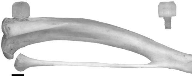
**Figure 4:** Rat tibia with inserted PMMA screw and loose PMMA screw. The internal portion of the screw has the same measurements as the stainless steel screw used for pull-out experiments. (Scale bar 3 mm)
